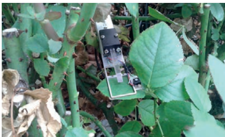
Figure 1 Micro-moni-PAM sensor (Gademann Instruments GmbH) placed in a leaf of a rose plant during the experiment.
