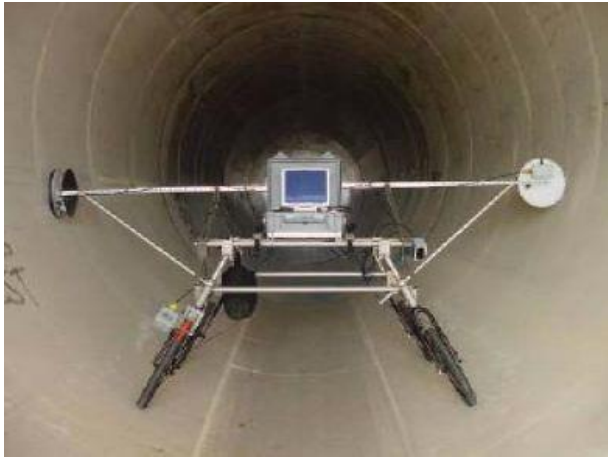
Figuur 9 P-Wave elektromagnetisch meetinstrument (Pure Technologies)
