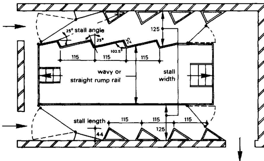
Fig. 6 Plan of a double four herringbone parlour with on one side a wavy rump rail with wavy pit edge and on the other side a straight rump rail with straight pit edge.
