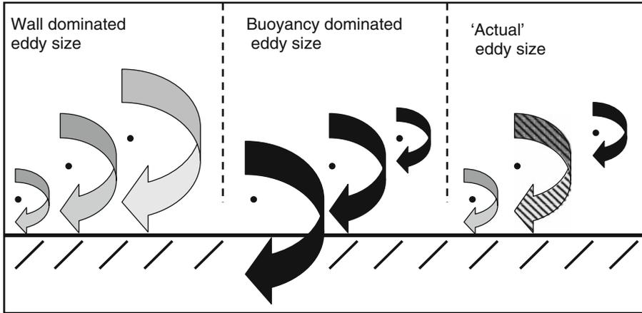
**Fig. 3** ‘Actual’ maximum eddy size as a combined result of wall (grey) and buoyancy (black) effects. In the first two frames *virtual* eddies are drawn. Note that the virtual, large eddy in the second frame only indicates that buoyancy is non-limiting near the ground. The actual eddy close to the ground is limited by wall effects (grey eddy, third frame). The dashed eddy is limited by both wall and buoyancy effects
