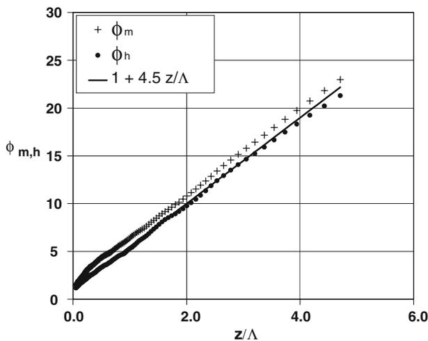
**Fig. 1** Dimensionless gradients as a function of the stability parameter  $z/\Lambda$ , as obtained from DNS (see: Appendix A). For comparison the line  $\phi_{m,h} = 1 + 4.5z/\Lambda$  is given
