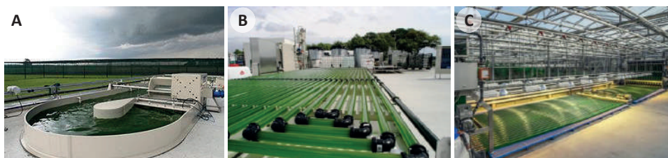
Figure 8.2 Different systems used in microalgal cultivation. (A) Open raceway ponds. (B) Photobioreactors. (C) Photobioreactor inside a greenhouse.
