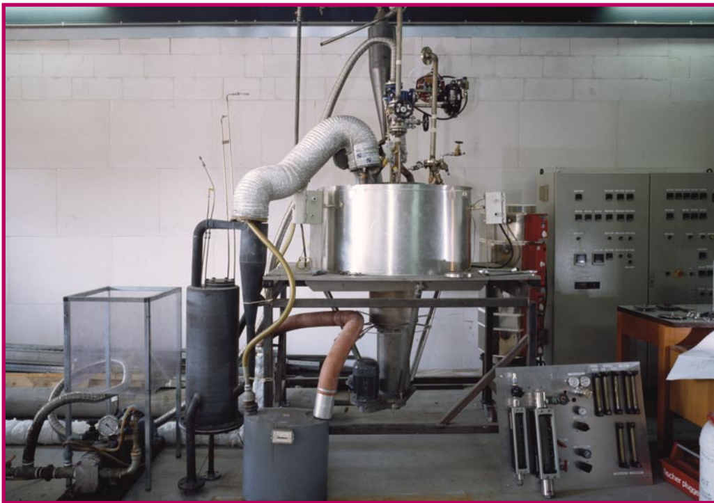
Trial installation for pyrolysis at the Biomass Technology Group B.V. te Enschede
