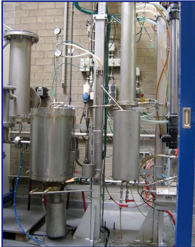
Pyrolysis test installation, University of Twente (photograph and copyright: Webletters, Anne Groot)
