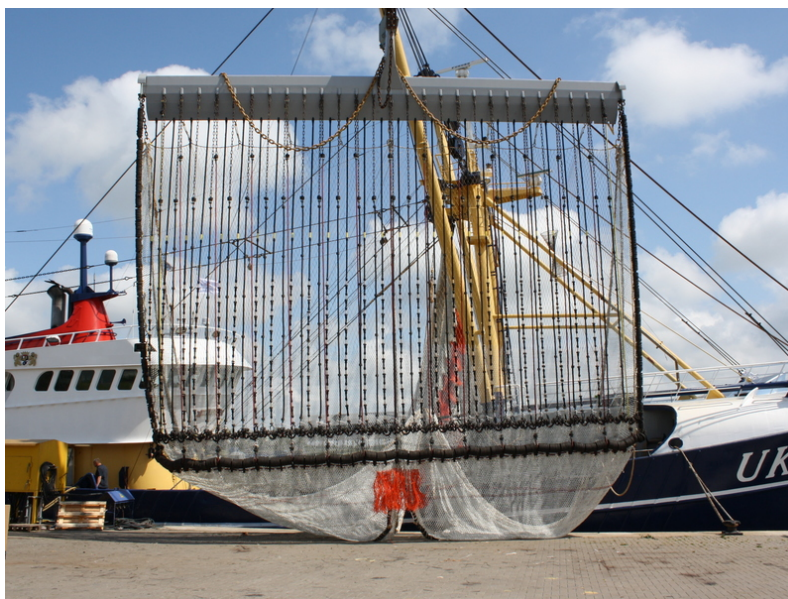
Figure 3. Pulse trawl fishing gear: The electrodes generate an electric pulse to catch flatfish.
