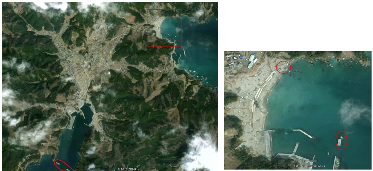
Figure 9: Left: Ryori bay after the tsunami. The severely damaged caisson breakwater and the sandy beach with the tsunami wall are designated; Right: Zoom in the tsunami wall bay. The large breakage on its north end, and the severe damage of the caisson breakwater are noted (Google Earth images, 2011)
