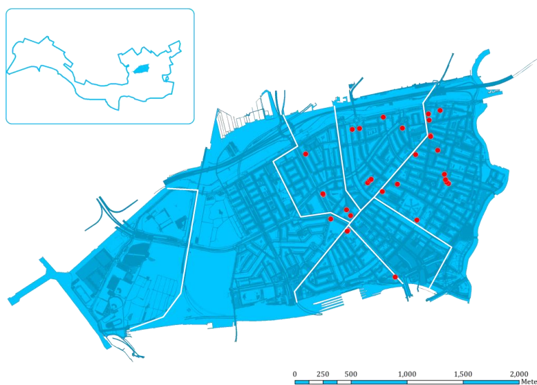
Figure 2.11 Map of Rotterdam Noord, marking the buildings that will flood at least once every two years (Veerbeek and Husson, 2013). NB: this is a Proof-of-Concept, not a substantiated vulnerability analysis.
