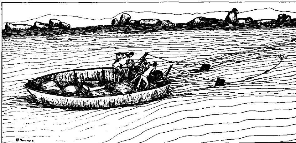
Figure 4.22 Shooting/hauling the bottom trawl of a small, outboard engine powered trawler.
