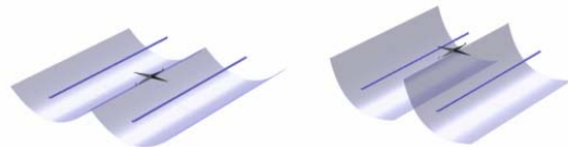
Fig. 4 Parabolic reflectors rotate in the East-West direction
