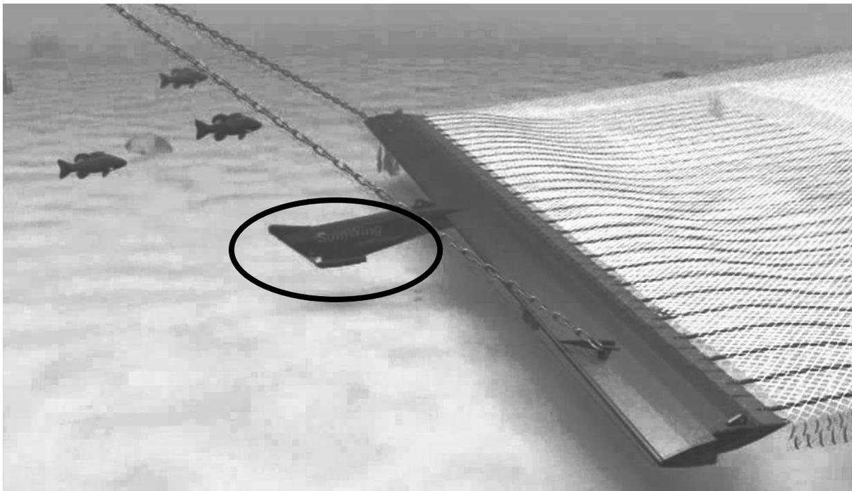
Figure 1: Graphical representation of a wing-type gear. Encircled is the nose of the gear which guards the wing from touching the seabed. (Illustration of sumwing developed by HFK Engineering)
