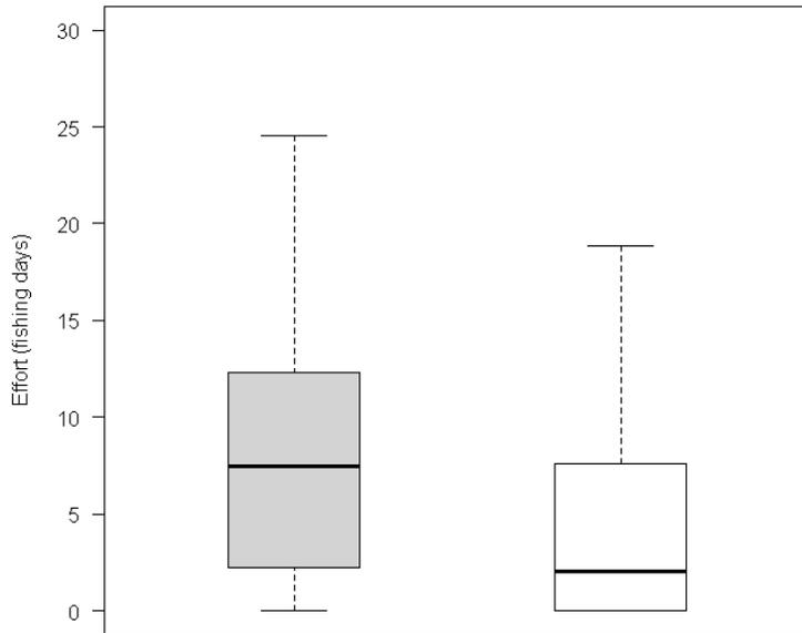
Figure 8. Effort as estimated at the breakpoint locations (shaded grey) and at random locations on the communication cables (white). Mean effort is given in a black solid horizontal line while the boxes indicate the 1<sup>st</sup> and 3<sup>rd</sup> quantile. The dashed lines indicate 1.5 times the 1<sup>st</sup> and 3<sup>rd</sup> quantile distances.
