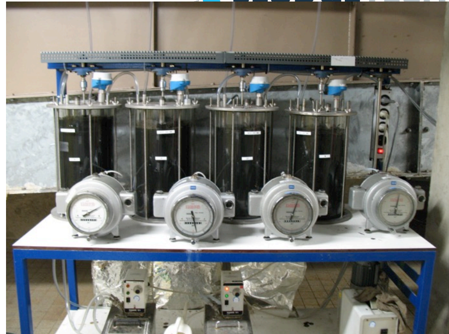
Digestion of treated sludge
