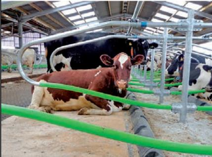
Wilson Agri says it has designed a cubicle system that reduces injuries caused by cows leaning and rubbing against steel when lying down. It is either post or floor mounted while supports and brackets are all made from galvanized steel. But the difference with the Cowcoon is that the bottom of the stall loop is replaced by a polyethylene tube. It has been designed to maximise cow
