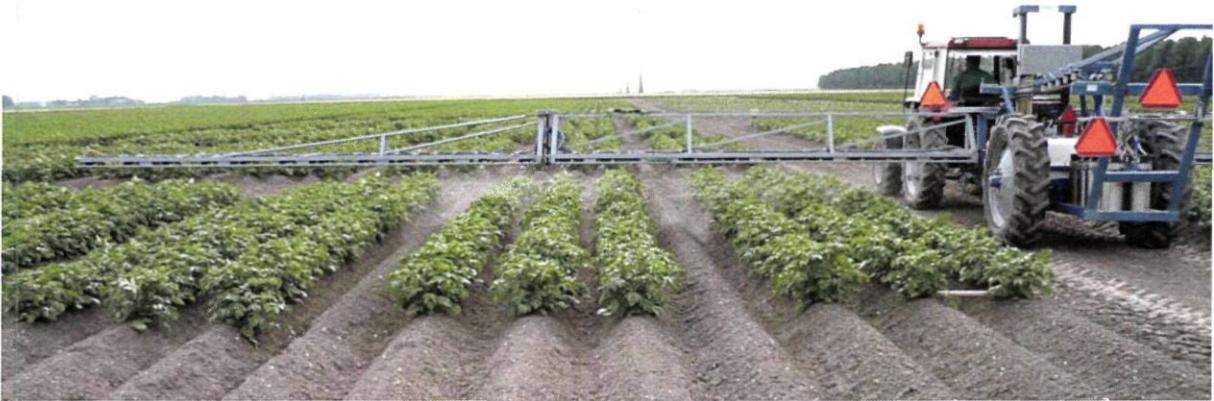
Figure 1: One of the beams of the Sosef-trial-spraying machine (in another experiment).
