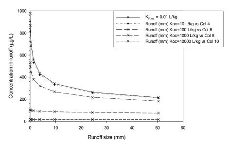
**Figure 6.2.1** Runoff water (mm per day) as a function of daily rainfall (mm, upper graph) and runoff concentrations ( $\mu$ g/L) as a function of runoff size (mm) and  $K_{oc}$  value (L/kg, lower graph) for maize with a RCN of 91 in the FOCUS runoff R2 and R4 scenarios
