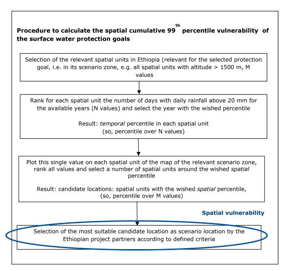
Figure 7.2.1 Schematic overview of the steps needed for selecting the scenario locations for the surface water protection goals.
