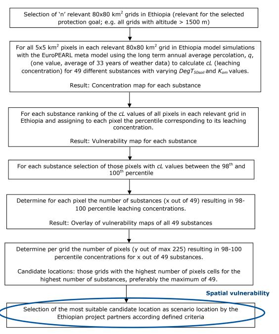
Schematic overview of the steps needed for selecting scenario locations for the Figure 7.1.1 groundwater protection goals.
