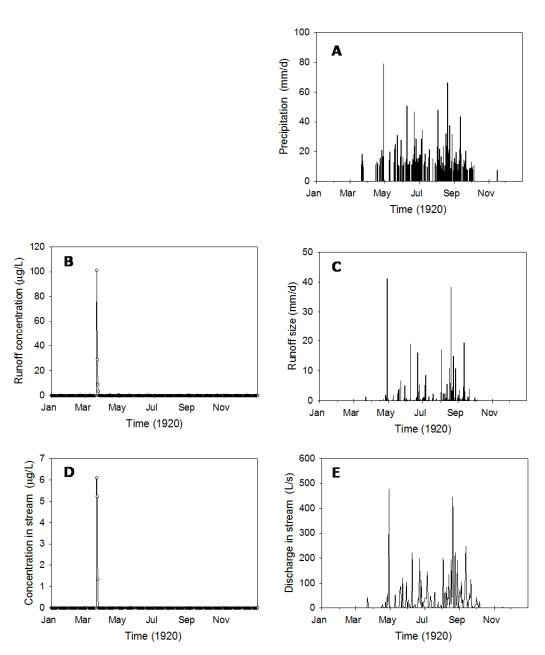
**Figure 13.3.2** Precipitation (A), runoff concentration (B), runoff size (C), concentration in the stream (D) and discharge in the stream (E) of grid 191 in the selected year 1920; results of simulations for one annual application of 1.44 kg/ha of 2,4-D in maize on 10 March.
