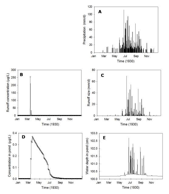
Figure 13.3.5 Precipitation (A), runoff concentration (B), runoff size (C), concentration in the pond (D) and water depth in the pond (E) of grid 217 in the selected year 1930; results of simulations for one annual application of 1.44 kg/ha of 2,4-D in maize on 10 March.
