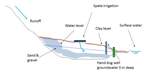
**Figure 5.2.3** Conceptual model of groundwater protection goal Alluvial aquifers at Rift Valley margins and in lowlands.
