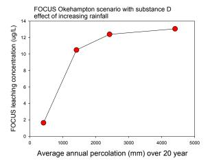
The FOCUS leaching concentration of FOCUS GW substance D (DegT<sub>50,soil</sub> =20 d at 20°C and Kom =35 L/kg at 20°C) as function of the average annual percolation over 20 year for the FOCUS groundwater scenario Okehampton.
