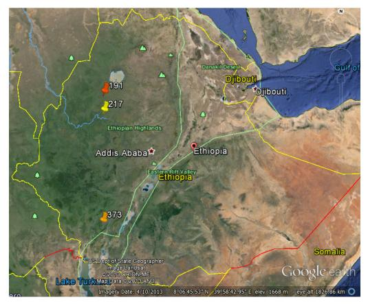
**Figure 8.2.1** Selected scenario locations for the surface water protection goals. Grid 191 for protection goal 1: Small streams above 1500 m, grid 373 for protection goal 2a Temporary ponds below 1500 m and with more than 500 mm rain and grid 217 for protection goal 2b Temporary ponds between 1500 m and 2000 m.
