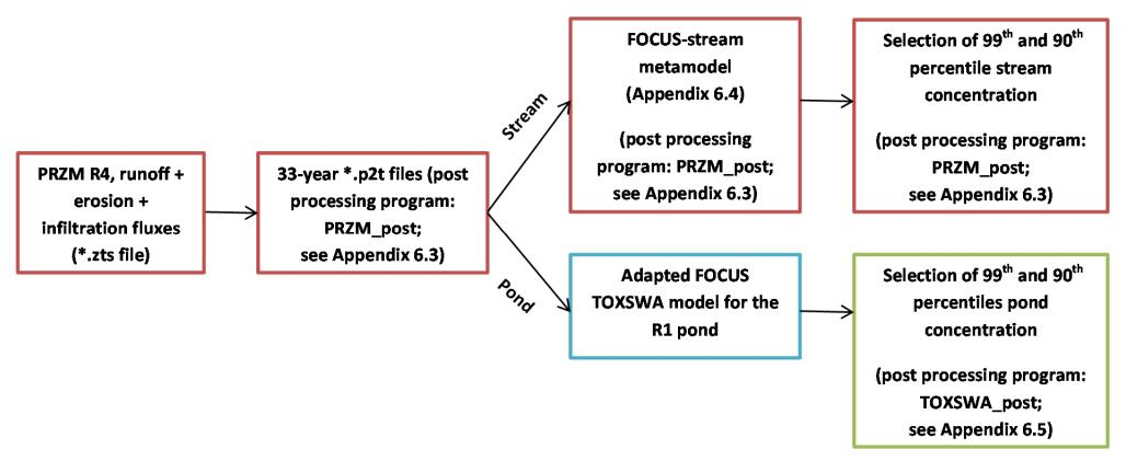
**Figure 9.2.1** Procedure for calculating the exposure target concentrations in the small stream and the temporary pond.
