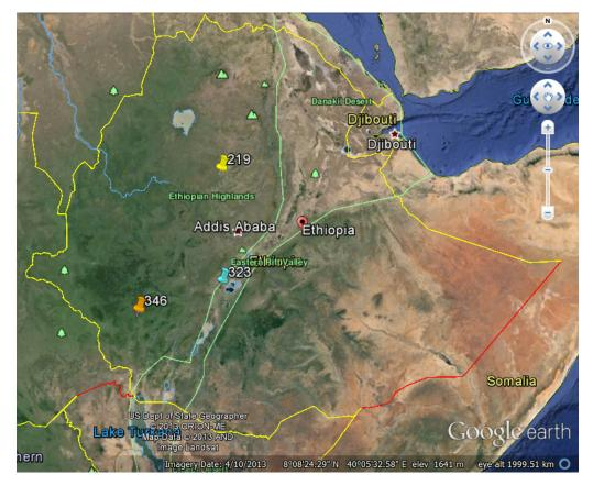
**Figure 8.1.1** Selected scenarios locations for the three groundwater protection goals. Grid 219 for goals 1 and 2: alluvial aquifers along small rivers and volcanic aquifers on shallow wells in areas above 1500 m; grid 346 for goal 3a: alluvial aquifers in the Rift Valley margins and lowlands below 1500 m altitude; grid 323 for goal 3b: alluvial aquifers in the Rift Valley margins and lowlands between 1500 -2000 m altitude.
