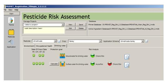
Screen shot of PRIMET\_Registration\_Ethiopia\_1.1 with an example project of Figure 14.1 dimethoate used on barley on the Drinking water tab, for assessment of risks for drinking water produced from groundwater and surface water.
