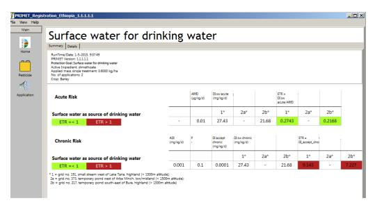
Figure 14.2 Screen shot of PRIMET\_Registration\_Ethiopia\_1.1 with an example project of dimethoate used on barley on the Drinking water tab. Results of the risk assessment for drinking water produced from surface water are shown for the three specific protection goals: the small streams above 1500 m altitude (1) and the temporary ponds below and above 1500 m altitude (2a and 2b).
