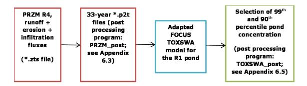
Figure A12.1 Flowchart of the procedure for calculating the exposure endpoints in the temporary ponds.
