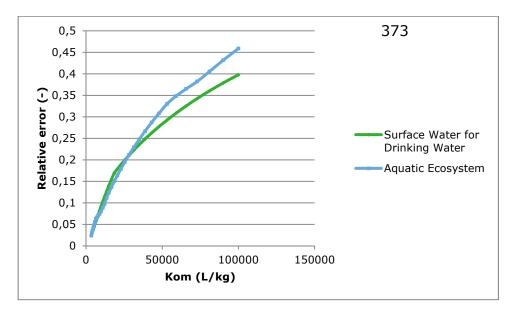
Figure A12.2 Relative differences according to equation 1 as a function of  $K_{om\_sediment}$  values for location 373 and the exposure endpoints for surface water for drinking water (green line) and aquatic ecosystem (blue line).
