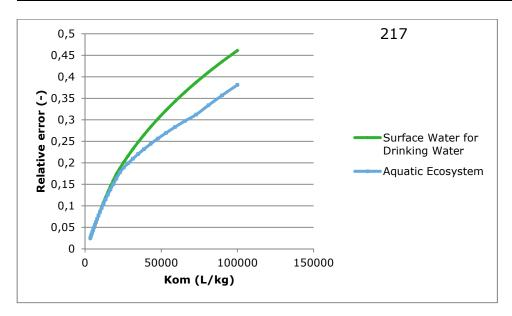
Figure A12.4 Relative differences according to equation 1 as a function of  $K_{om\_sediment}$  values for location 217 and the exposure endpoints for surface water for drinking water (green line) and aquatic ecosystem (blue line).
