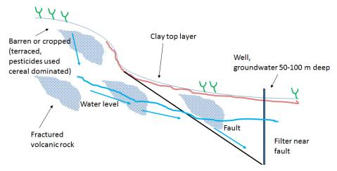
Figure 5.2.2 Conceptual model of groundwater protection goal Volcanic aquifers on shallow wells.
