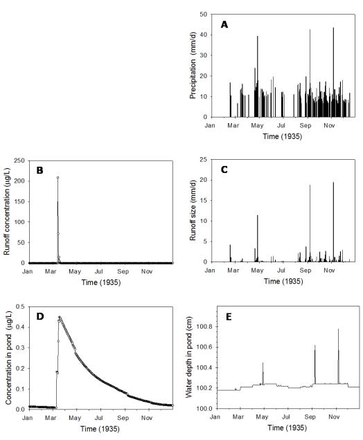
**Figure 13.3.4** Precipitation (A), runoff concentration (B), runoff size (C), concentration in the pond (D) and water depth in the pond (E) of grid 373 in the selected year 1935; results of simulations for one annual application of 1.44 kg/ha of 2,4-D in maize on 10 March.
