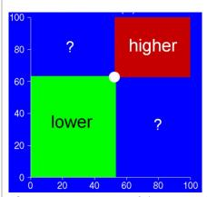
Diagram of the percentile of a stochastic variable z which is a function of two variables x and y. The horizontal axis consists of percentiles of x and the vertical axis consists of percentiles of y. It is assumed that z increases continuously as a function of x and y. The point in the plane is an arbitrary combination of x and y percentiles.
