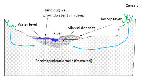
Figure 5.2.1 Conceptual model of groundwater protection goal Alluvial aquifers along small rivers.
