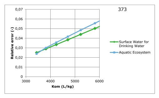
Relative differences according to equation 1 as a function of  $K_{om\_sediment}$  values Figure A12.3 (detail) for location 373 and the exposure endpoints for surface water for drinking water (green line) and aquatic ecosystem (blue line).
