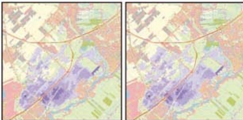
Figure 1: Illustration of inundation simulation after a breach in the dike of the Hollandsche IJssel near Moordrecht (Deltares)
