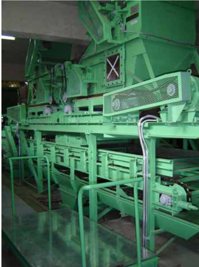
Figure 39 The mat former, showing the mixing section and the transportation section for the carrier sheet
