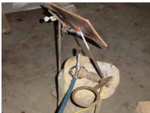
Figure 31 Set-up of fire resistance test at FPRDI.
