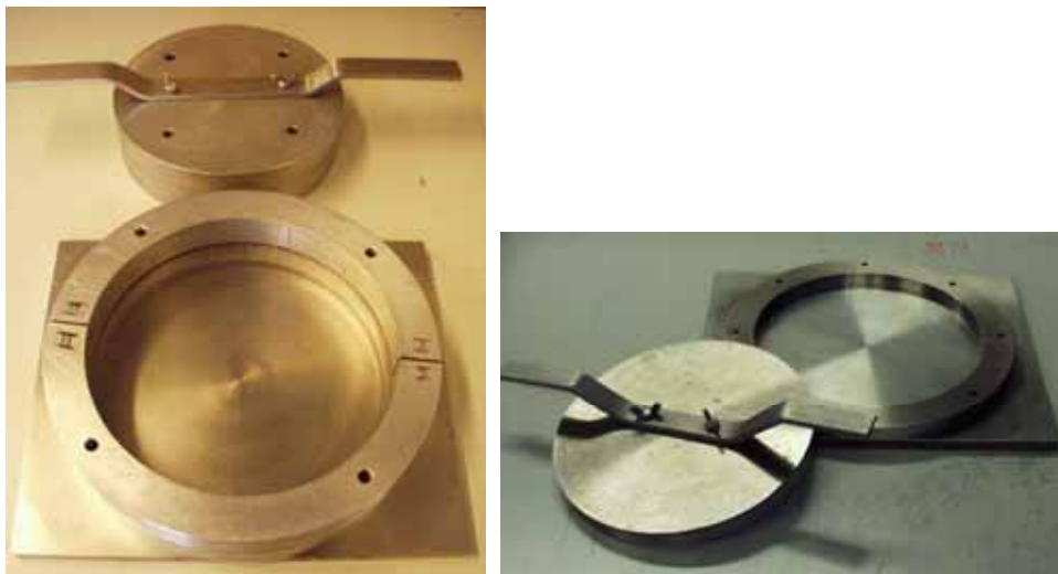
Figure 1 Photograph of mould in which husk is hot pressed.
