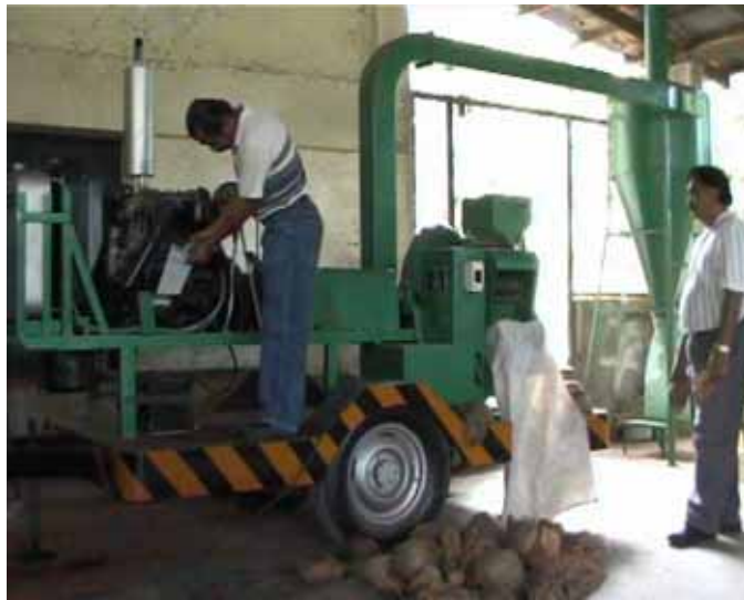
Figure 45 Pilot cutting mill, specially designed for milling coconut husk for application in panel boards.
