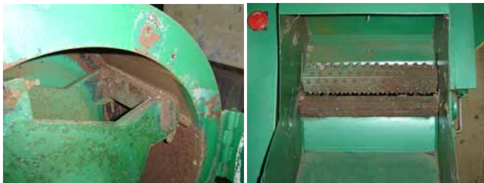
Figure 34 The milling chamber before rehabilitation (a) and the feeder section (b)
