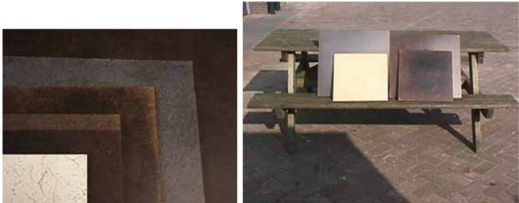
Figure 26 Photograph of boards pressed. Left picture, from bottom-left to right: 5, 4, 3, 1 and 2. Right picture shows the relative dimensions in front of a garden seat+table.
