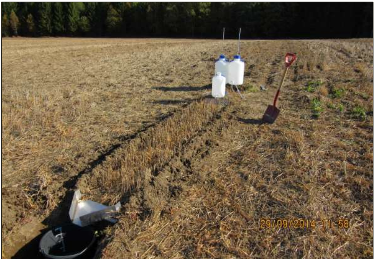
FIGURE 8: THE MEASUREMENT SET UP SHOWING THE PLOT BOUNDED BY TWO SMALL WALLS, THE MARIOTTE BOTTLES, THE FLUME, AND BUCKET.
