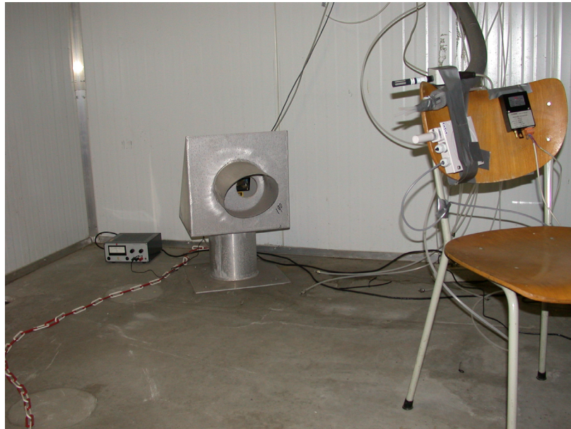
Figure 2.6 Boreal TDL, Viasala ammonia sensor, Rotronic and pressure sensor inside the controlled chamber
