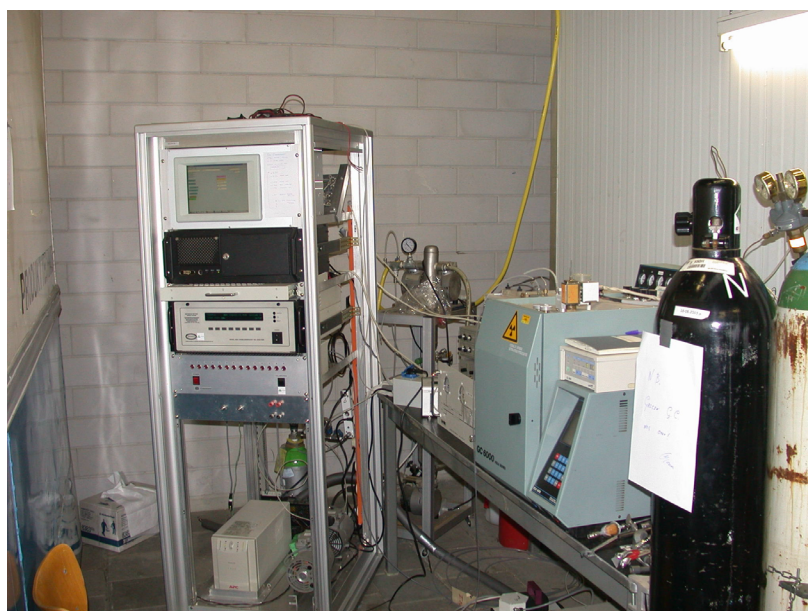
Figure 2.5 Reference instruments for the experiments; Converter with \text{NO}_x monitor and data acquisition system (rack), gas chromatograph, air dilution system for \text{CO}_2 monitor (next to GC) and \text{CO}_2 monitor (just visible)
