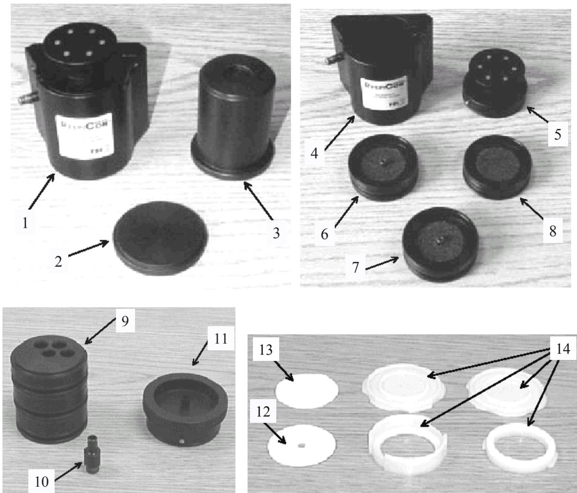
Figure 1 RespiCon sampler. 1: RespiCon sampler; 2: Removal lid; 3: Removal cylinder; 4: RespiCon body unit; 5: Inlet head; 6-8: filter stages; 9: Stage flow checker; 10: Stage flow checker inlet; 11: Total flow checker; 12: 37-mm filter with hole; 13: 37-mm filter without hole; 14: Filter cassette (shown disassembled) with top and bottom lid
