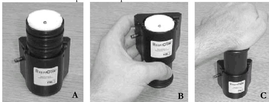
Figure 6 Assembling the RespiCon Particle Sampler
