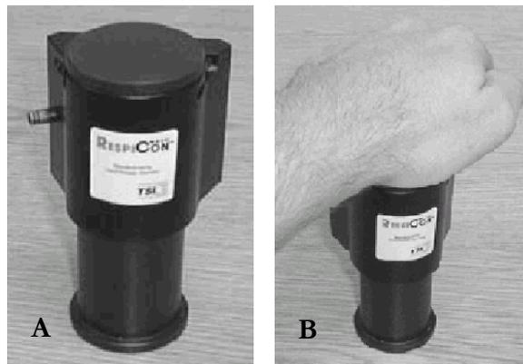
Figure 5 Disassembling the RespiCon Particle Sampler
