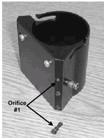
Figure 4 Orifice location, orifice #1 shown removed
