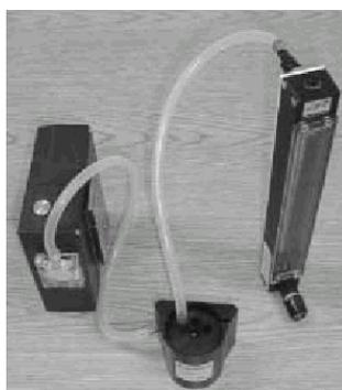
Figure 3 Attach flowmeter and sampling pump to RespiCon stage flow checker
