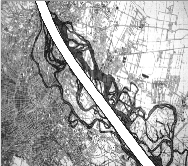
Fig. 1. River regulation, starting in 1875, of the Danube at Vienna. The graph shows the original braided river system and the constructed single channel.
