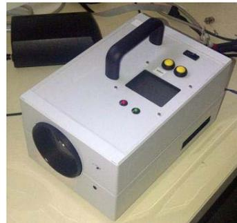
Ripeness sensor based on fluorescence measurement (Force-A)
