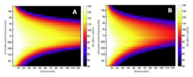
Figure 18. Predicted 1/3 octave band spectrum of the sound exposure level (SEL) at 1-m above the seabed, as a function of distance from Luchterduinen tower 28, during a single pile-drive at an energy level of 1400 kJ: A) with no wind interference; B) with wind at 6-8 m/s, creating noise on the surface that reduces sound propagation. Figure taken from de Jong et al. (2013).
