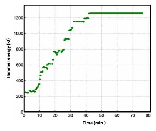
Figure 7. An example of the change in energy level and frequency of blows over time during pile-driving of a turbine tower. This is a scenario based on a total of 2500 hammer blows and a maximum energy of 90% of 1400kJ. Figure adapted from de Jong et al (2013).
