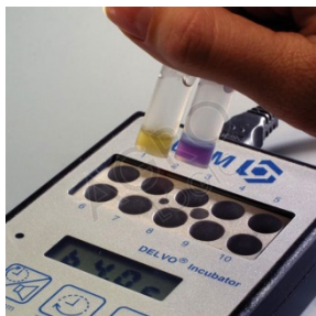
Figure 4 DelvoTest ® , negative sample on the left (yellow) and positive sample right (purple).
