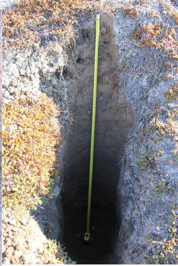
Figure 37: Picture of soil pit J11, located in the colluvium captured by the highest terrace ridge. The thick cover of fine material is located on top of the beach deposits. Some gravel is captured in the 1A horizon.
