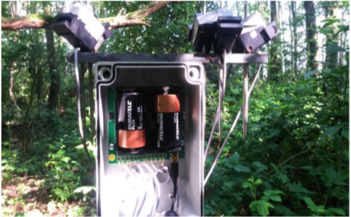
Figure 2.3.: PASTIS57 instrument during the field campaign. The front cover is removed and the six sensors are mounted on top oriented to different azimuth angles.
