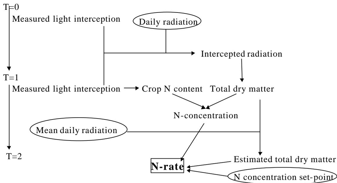
Fig. 2. Lay out of system for supplementary N application based on the measurement of light interception
