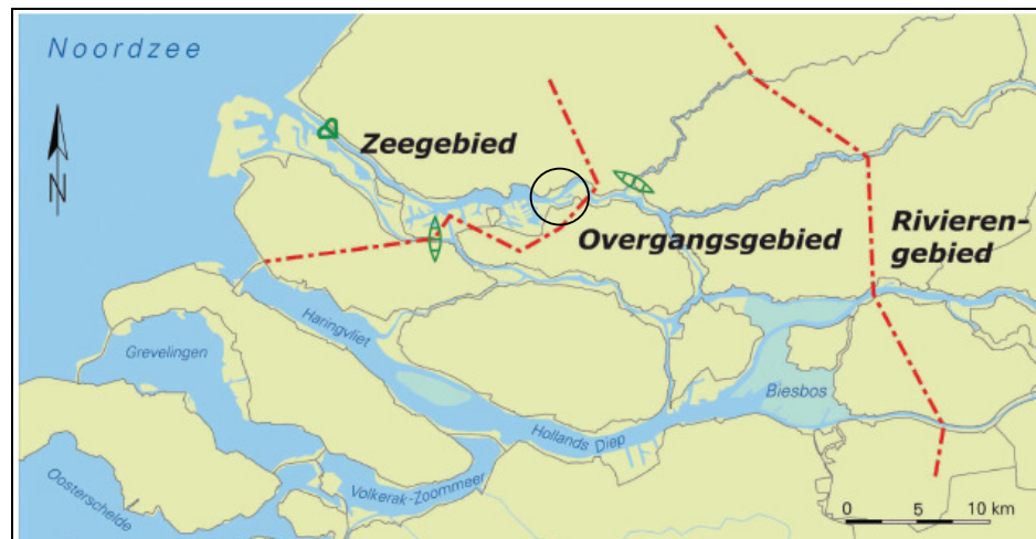
Figure 9.1 Influence of sea levels and/or river discharges on river water levels (J.P. de Waal, 2007). The water levels in the 'Rivierengebied' (river area) are the result of the river discharges, in the area 'Zeegebied' (sea area) the water levels are determined by the sea levels and in the 'Overgangsgebied' (transition zone) both the river discharge and the sea levels influence the water levels. The study area is located within the circle.
