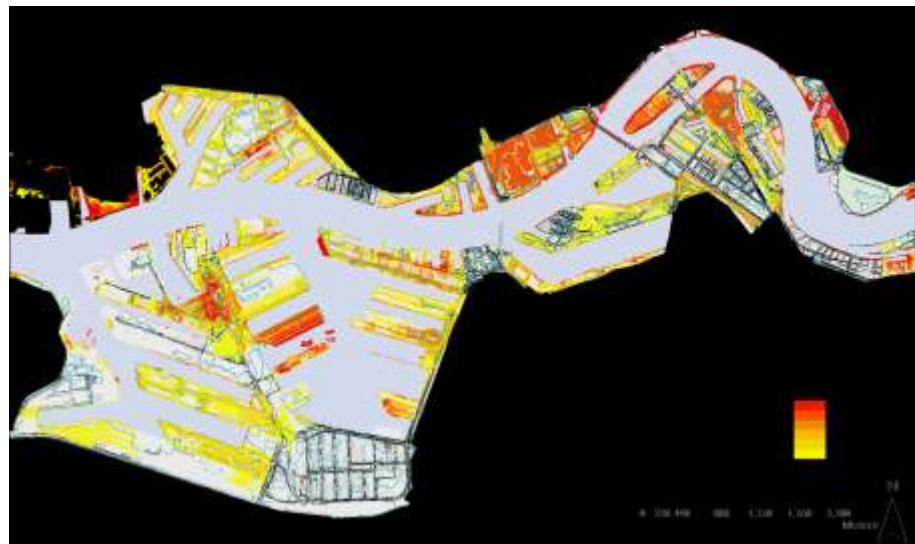
Figure 2: flood extent associated with the predicted return periods for the current conditions in the Rotterdam unembanked area.
