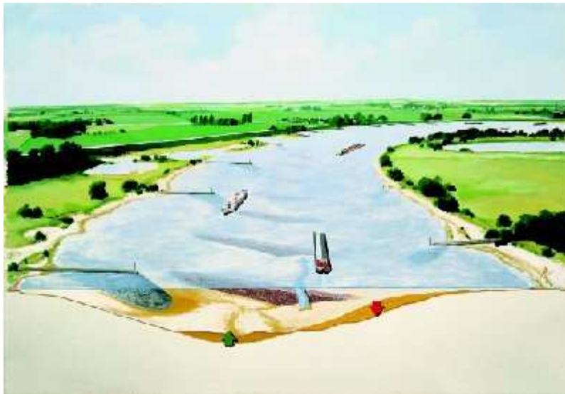
Figure #.2. Bendway weirs in outer-bend pool.
