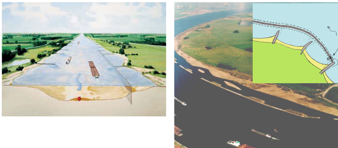
Figure #.4. Longitudinal dams (example in right panel: Parallelwerk Walsum-Stap, Germany).
