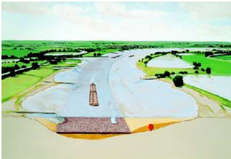
Figure #.13. Fixed layers to correct the cross-sectional profile in bends of the river Waal.
