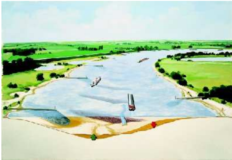
Figure #.12. Bendway weirs to correct the cross-sectional profile in bends of the river Waal.
