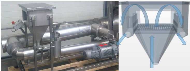
Figure 1. Left: Pilot cross-flow frying unit with pump, heating unit and frying section. Right: Frying section with oil entering from below, flowing via a perforated plate into the bath, and leaving the system via the sides.
