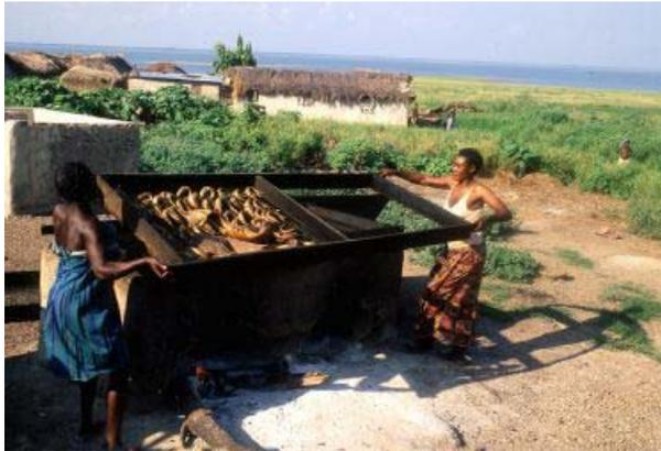
*Figure 7 Preparing fish for smoking on a Chorkor oven
