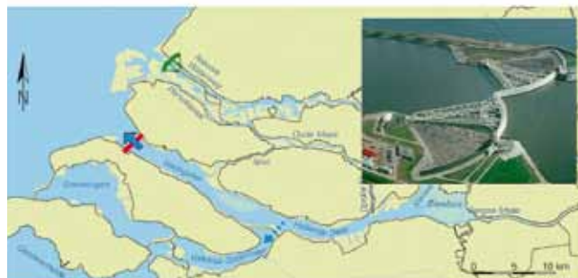
Fig. 1. Protection of unembanked area in Rijnmond-Drechtsteden by 1) higher elevation of ground (man made), 2) storm surge barrier (only the Maeslantkering is shown)
