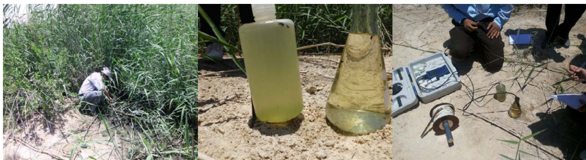
Photo 12 Sample taken from wetland below weeds and measuring field parameters using WTW multi 350i device (EC, pH, dissolved oxygen and temperature).
