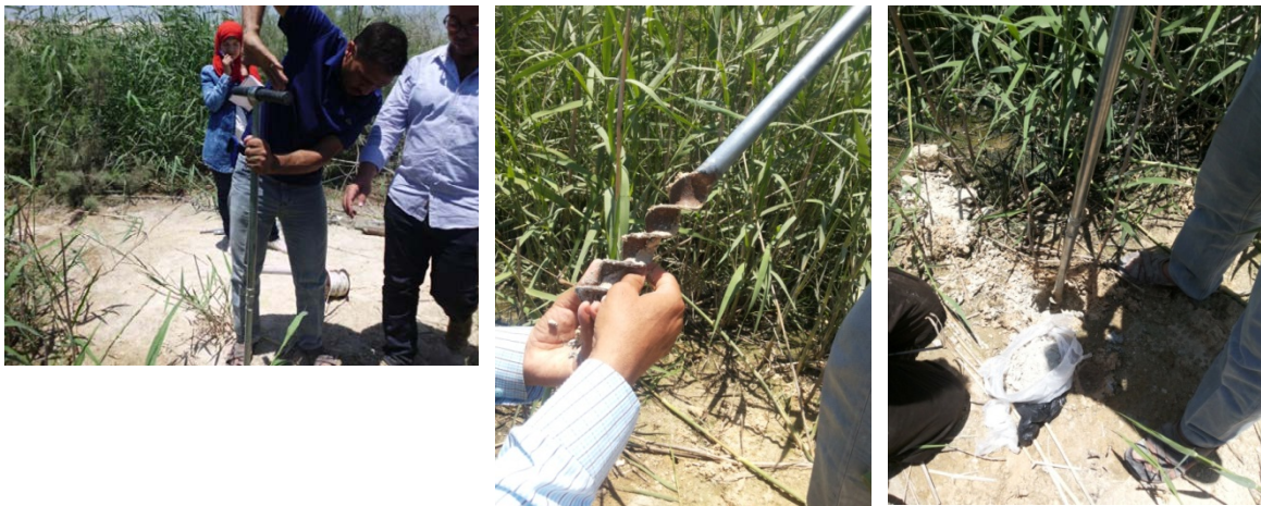
Photo 14 Hand auger drilling and collection of soil samples
