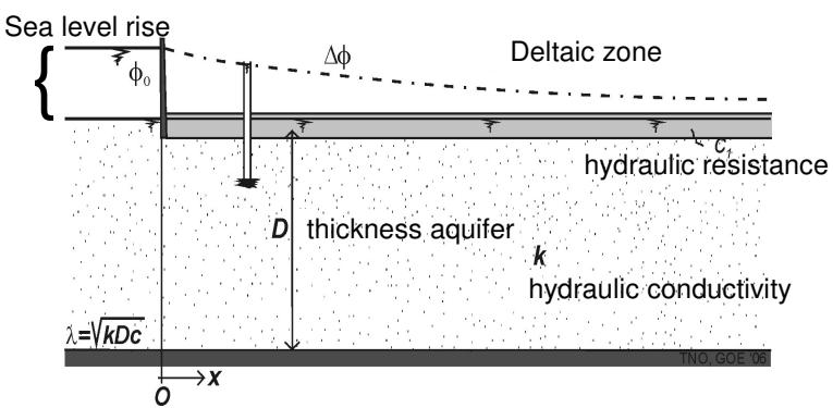
Sea level rise  $\phi_0$ , Deltaic zone, hydraulic resistance  $c_t$ , thickness aquifer  $D$ , hydraulic conductivity  $k$ ,  $\lambda = \sqrt{kDc}$
