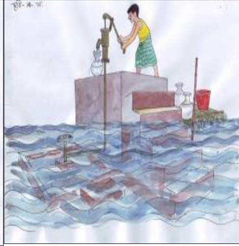
Raised and normal combined platform during flood
