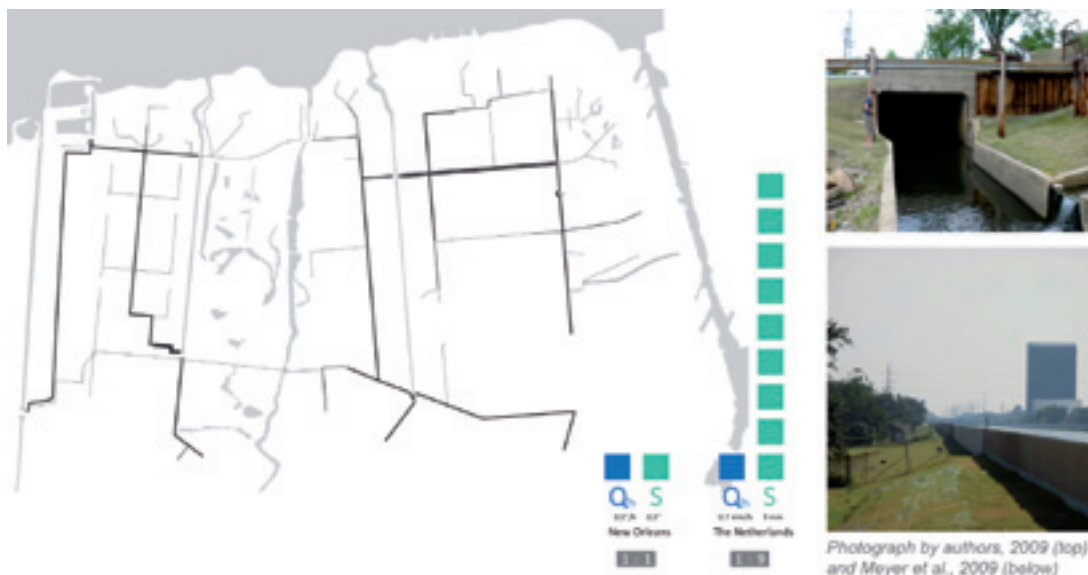
Figure 7 Technocratic watermanagement: subsurface drains, deep drainage regime, discharge dependend system, floodwalls. (Sewerage and Water Board of New Orleans, unknown date; Hooijmeyer et al., 2005; USACE, 2009)
