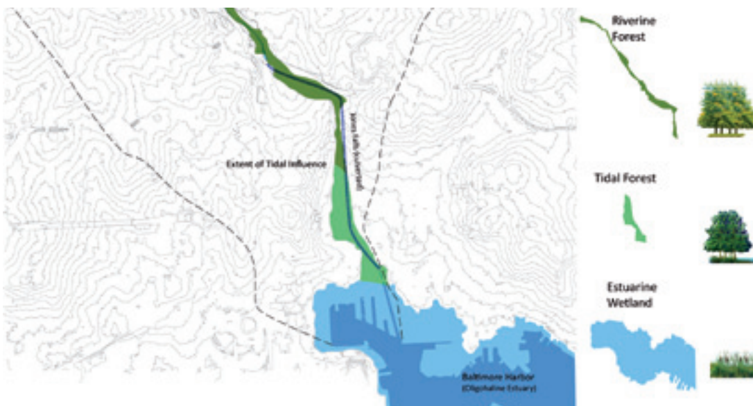
Figure 3 The city's physiographic armature suggests three specific ecological zones along the JFX corridor: the riverine forest, the tidal forest, and the estuarine wetland. Fluctuating water levels are characteristic of the dynamics of these communities. The culvert currently suppresses this fluctuation, thereby suppressing the specific qualities of the city's regional setting..
