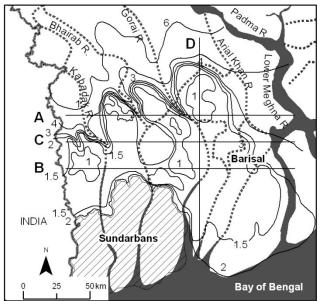
Figure 4. Contours of elevation are in mPWD based on the DEM of the 1950s and the river courses based on the 1943 map are shown by dashed line
