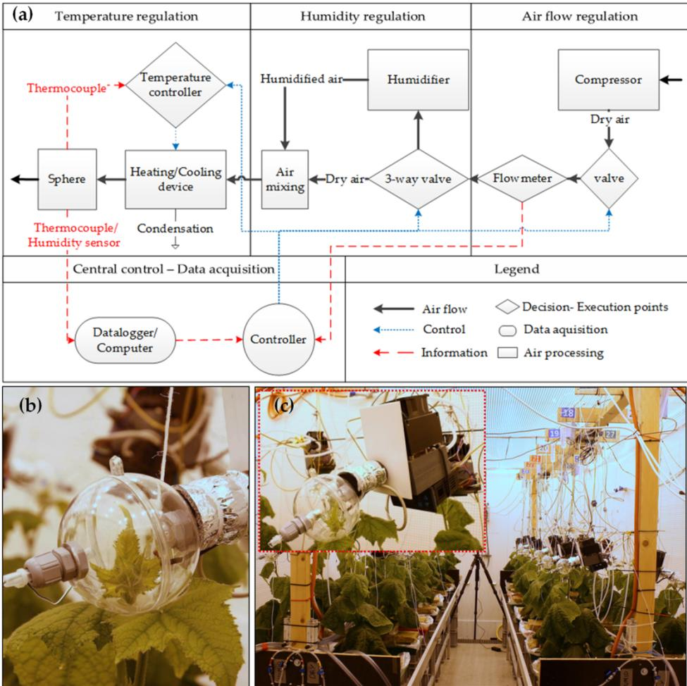
**Fig. 1.** Schematic representation of the heating/cooling system used to alter apical bud temperature in cucumber plants (a). Transparent sphere used to isolate apical bud from the ambient environment (b). Experimental setup in the climate room and a magnified image of one of the heating/cooling modules attached on a cucumber plant (c).
