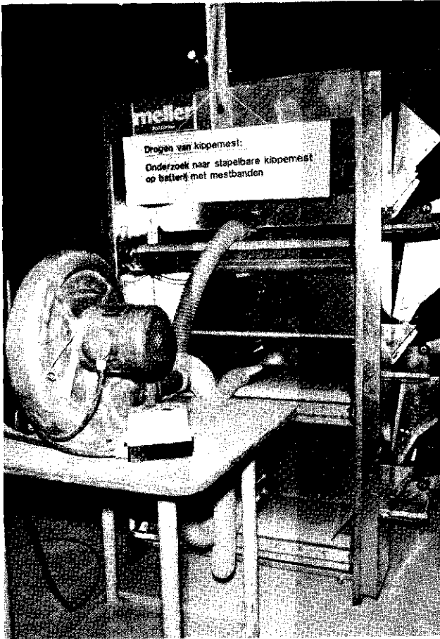
Fig. 1. Prototype set-up for drying manure in batteries
