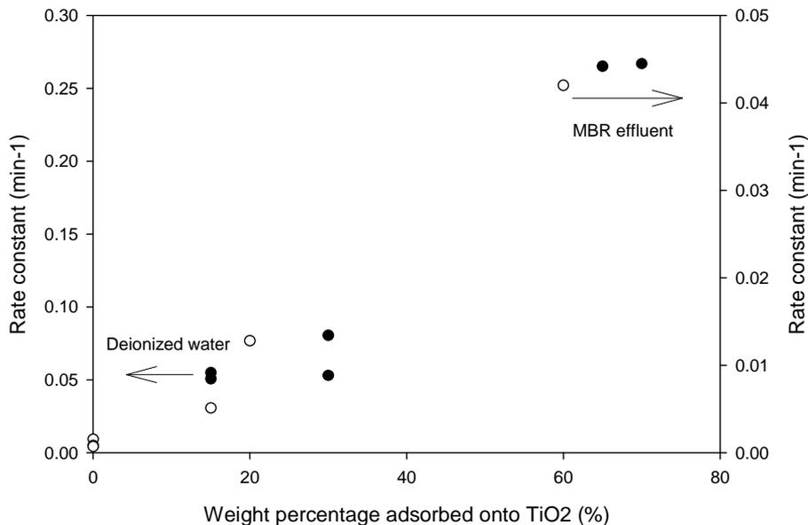
Figure 7.5: Rate constant as a function of weight percentage adsorbed onto TiO<sub>2</sub>, solid symbols are deionized water and open symbols MBR effluent .
