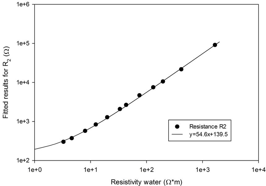
Figure 3.7: Fitted results of  $R_{C_2}$  (glass beaker inductor) as a function of resistivity water.
