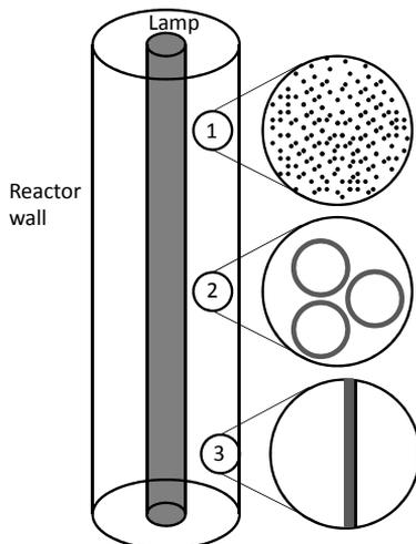
Figure 1.3: Annular photocatalytic reactor with 1) suspended photocatalyst, 2) immobilized photocatalyst on glass beads and 3) immobilized photocatalyst on the reactor wall.
