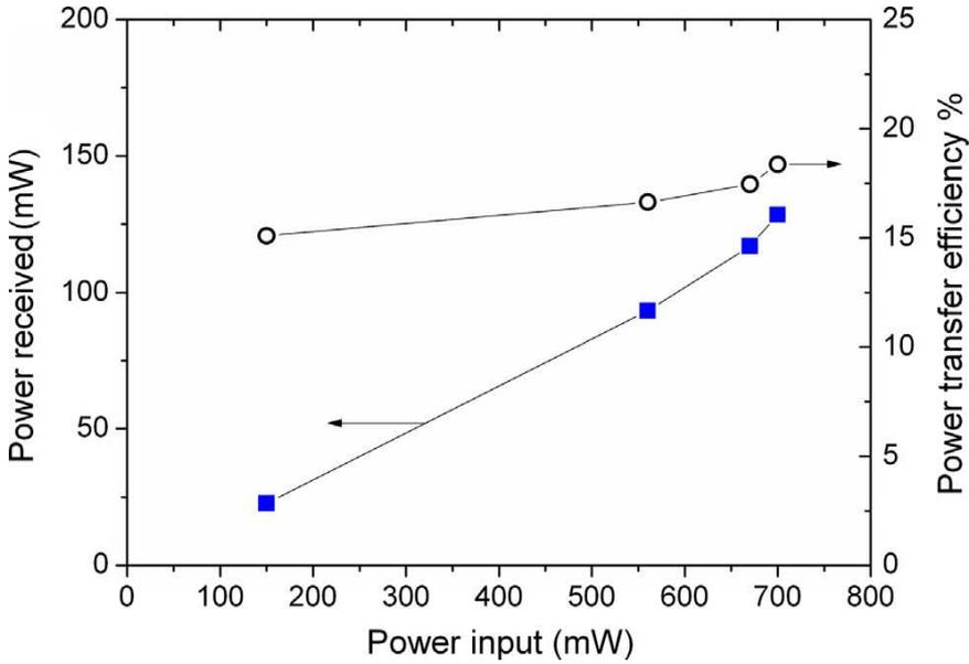
Figure 4.7: Power received at the load and the power transfer efficiency as function of the power input in the transmitting circuit.
