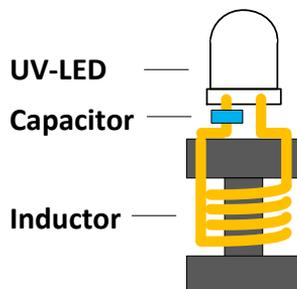
Figure 6.2: Schematic drawing of the receiving circuit with an inductor, capacitor and UV-LED.
