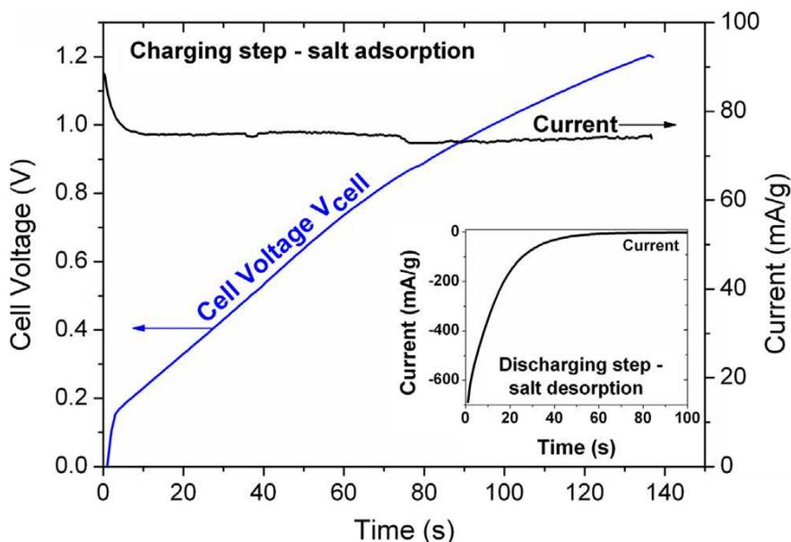
Figure 4.4: Experimental data for the cell voltage between the two porous electrodes of the wireless CDI design,  $V_{cell}$  (blue line), and current (black line) in one desalination cycle upon wireless energy transfer by resonant inductive coupling (RIC). Insert shows desorption step during which current flows in the opposite direction.
