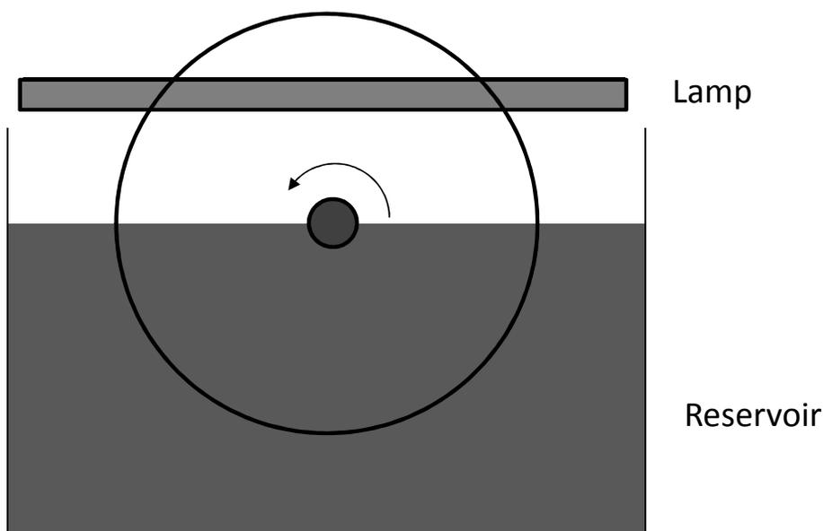
Figure 1.5: Schematic drawing of a vertical spinning disk reactor.
