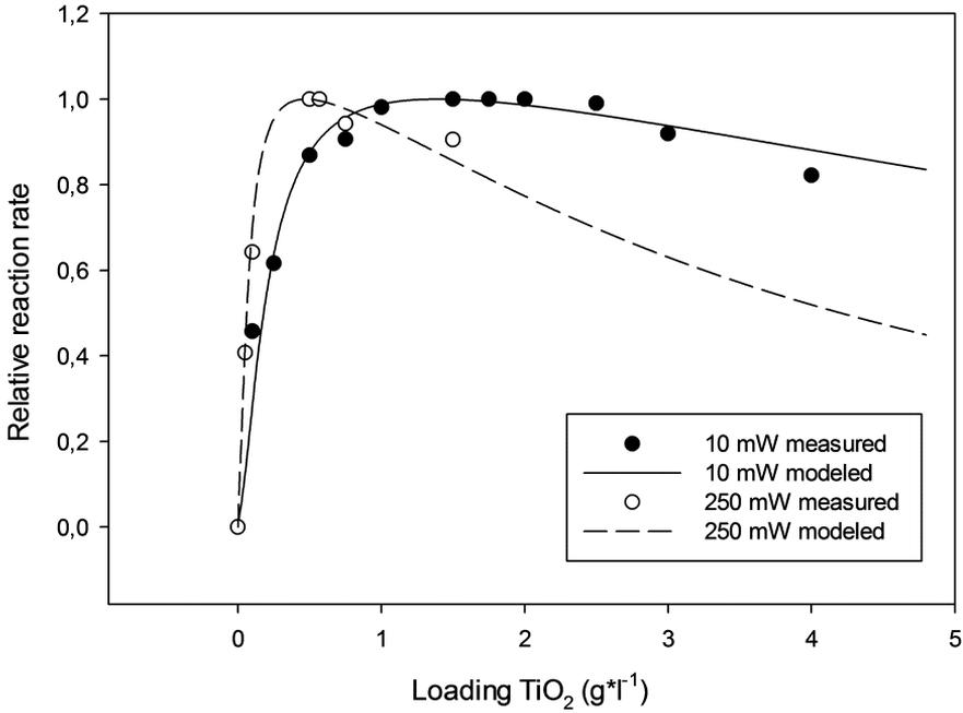
Figure 5.3: Relative reaction rate as function of TiO<sub>2</sub> loading measured and modeled with 10 and 250 mW radiant power UV-LEDs
