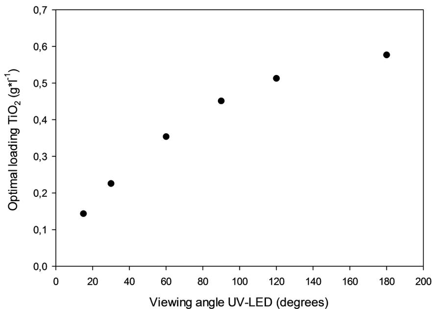
Figure 5.5: Optimal loading as function of emission angle of the 250 mW UV-LED
