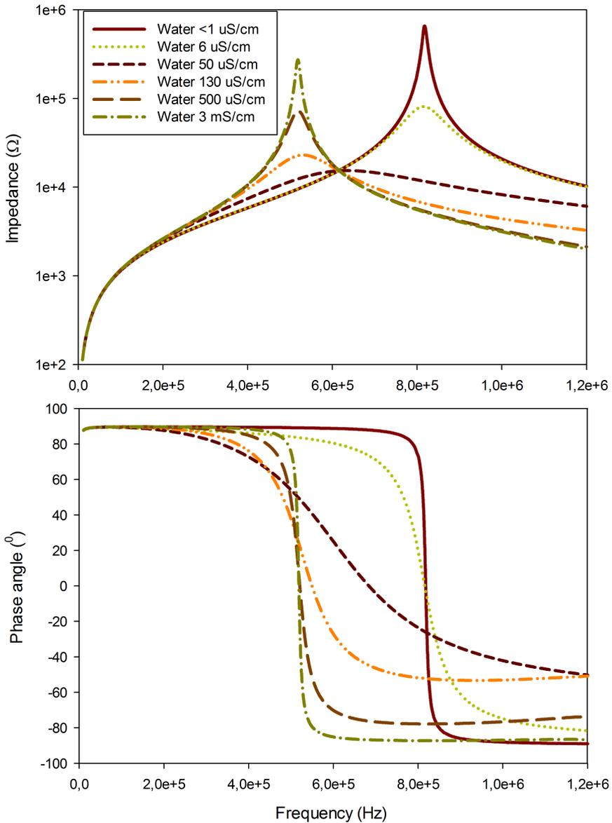
Figure 3.5: Impedance and phase angle as a function of frequency for inductor wound around the glass beaker, filled with water with different conductivities.
