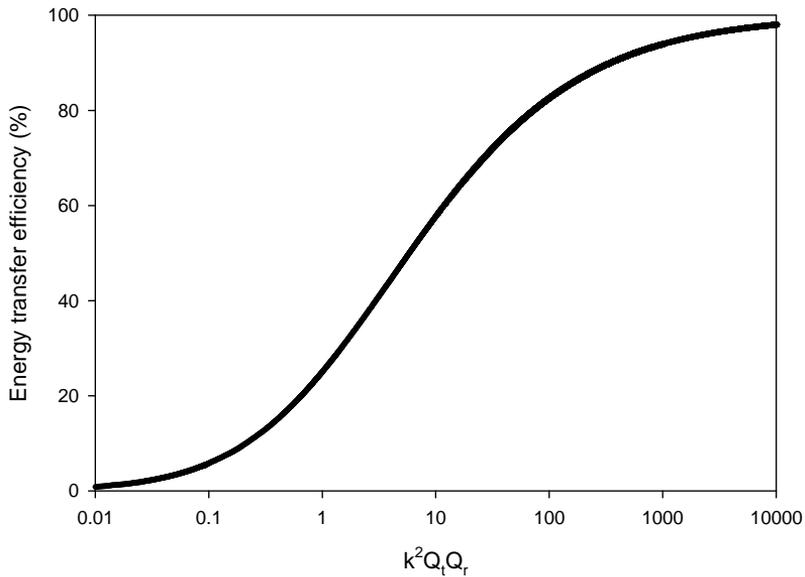
Figure 1.11: Energy transfer efficiency as function of  $k^2 Q_t Q_r$
