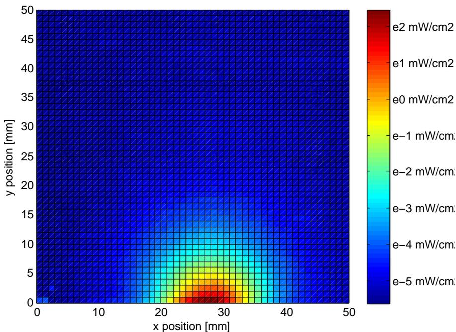
Figure 6.6: Measured light intensity of a 10 mW radiant power UV-LED irradiating into a  $\text{TiO}_2$  suspension of 1 g/l.
