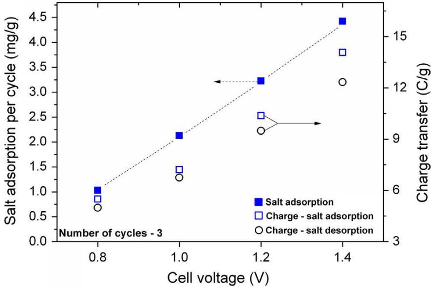
Figure 4.6: Experimental data of salt adsorption and charge transfer per cycle in wireless desalination, as function of maximum cell voltage difference,  $c_{salt} = 20$  mM, data given per mass of both electrodes.
