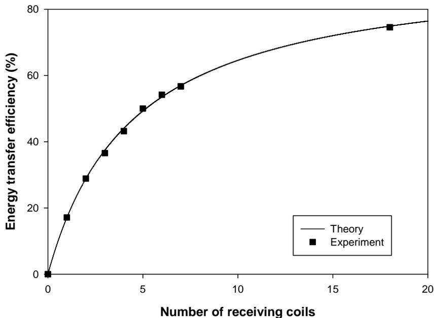
Figure 2.6: Energy transfer efficiency measured and calculated (Equation 2.1) between one transmitting inductor coupled to multiple receiving inductors.
