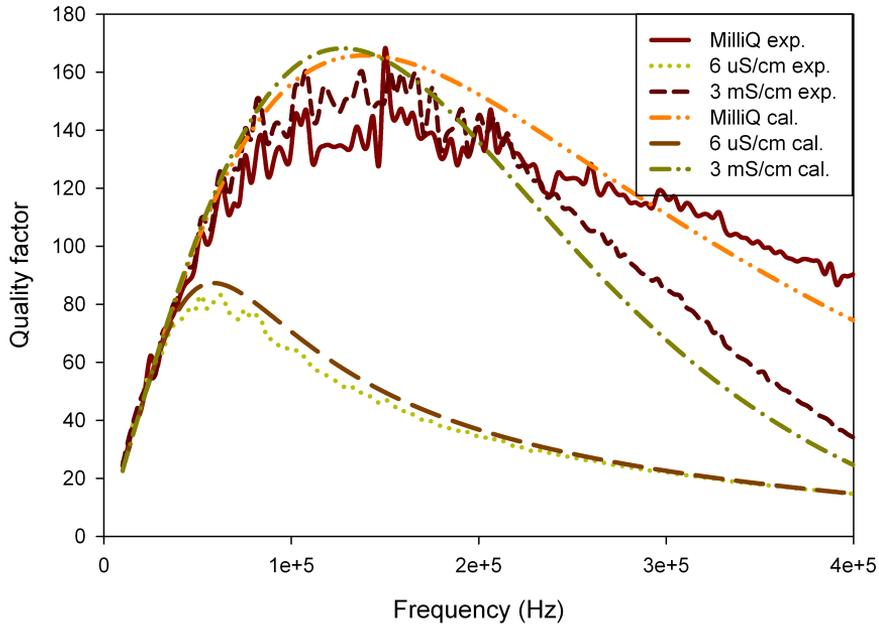
Figure 3.8: Quality factor as a function of frequency for the inductor wound around the glass beaker, measured and calculated with water with different conductivities.
