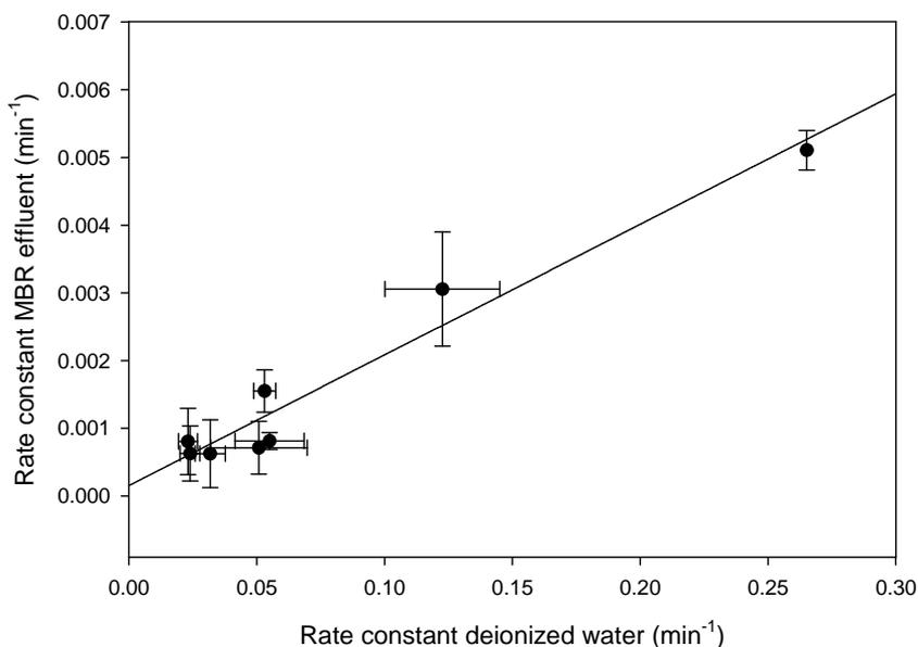
Figure 7.6: Rate constant for distributed UV-LEDs in MBR effluent as a function of the rate constant for distributed UV-LEDs in deionized water, error bars indicate 95% confidence interval.
