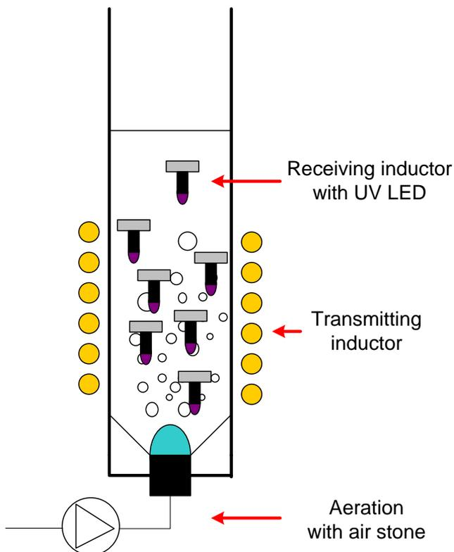
Figure 6.1: Schematic drawing of the photocatalytic reactor with aeration, transmitting inductor and the receiving inductor with UV-LED.
