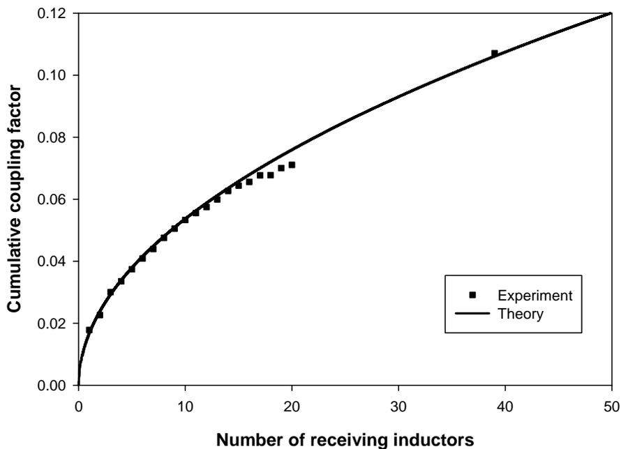
Figure 2.4: Cumulative coupling factor measured between one transmitting and multiple receiving inductors.
