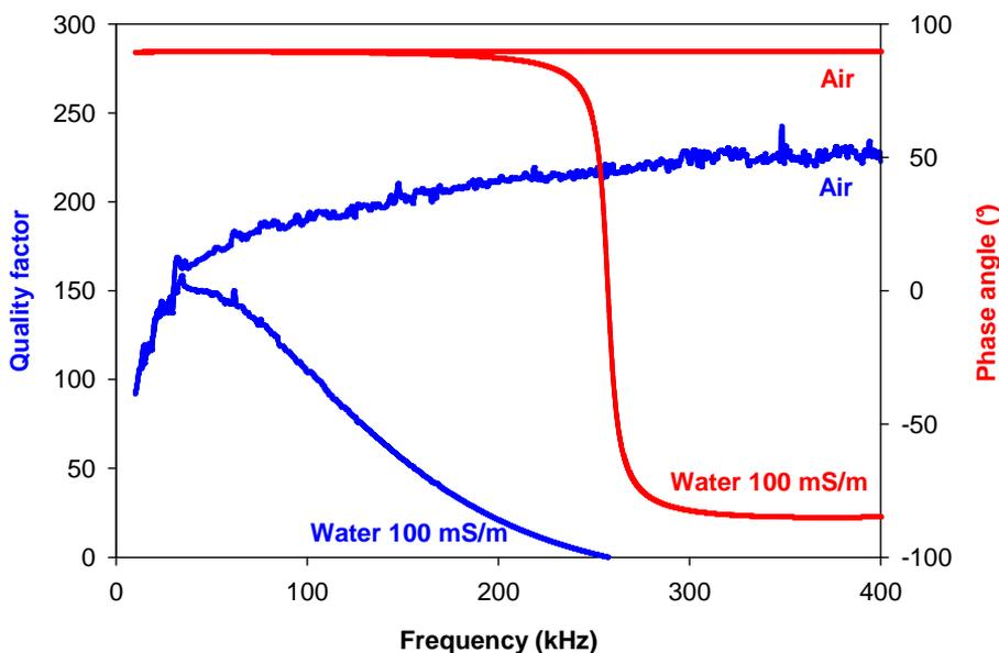
Figure 2.3: Quality factor and phase angle of transmitting inductor in air and filled with water with 100 mS/m conductivity.
