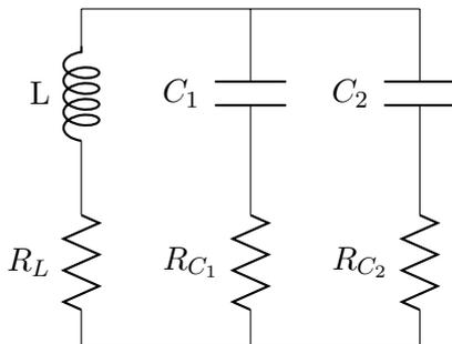
Figure 3.2: Lumped equivalent circuit of a water cored inductor, the inductance  $L$  (H) with series resistance  $R_L$  ( $\Omega$ ) and two parallel capacitances  $C_1$  and  $C_2$  (F) and two series resistances  $R_{C_1}$  and  $R_{C_2}$  ( $\Omega$ ).
