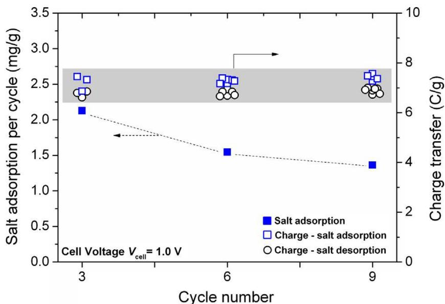
Figure 4.5: Experimental data of salt adsorption and charge transfer per cycle as function of total number of desalination cycles,  $c_{salt} = 20$  mM, data given per mass of both electrodes. Each desalination cycle consist of ion adsorption and desorption step.
