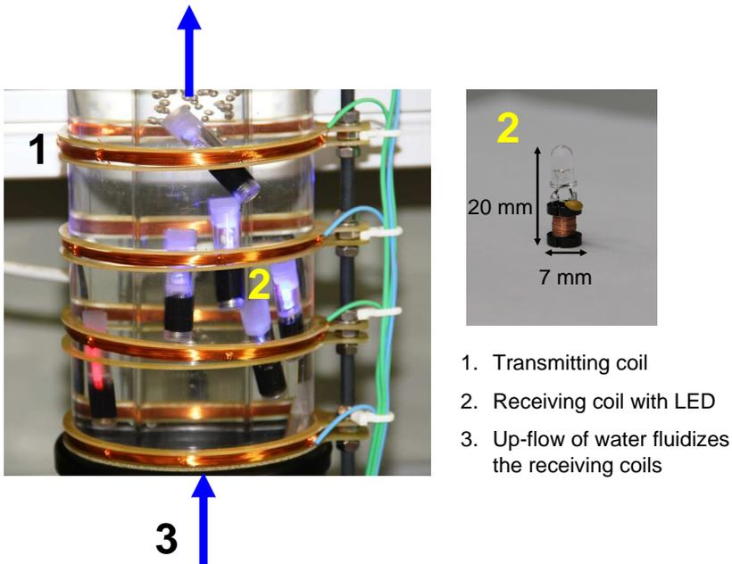
Figure 2.1: Demonstration of proposed water treatment system with dispersed LEDs powered wirelessly with inductive coupling.
