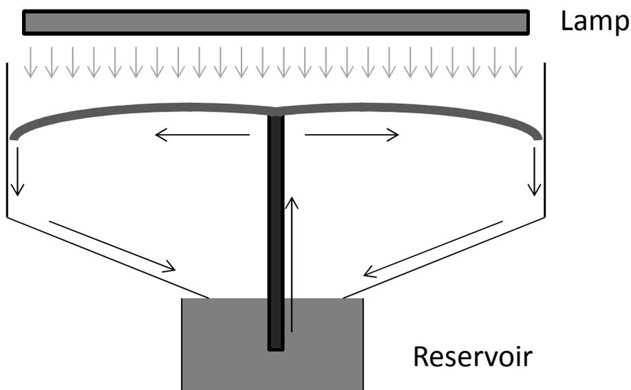
Figure 1.4: Schematic drawing of a fountain reactor.
