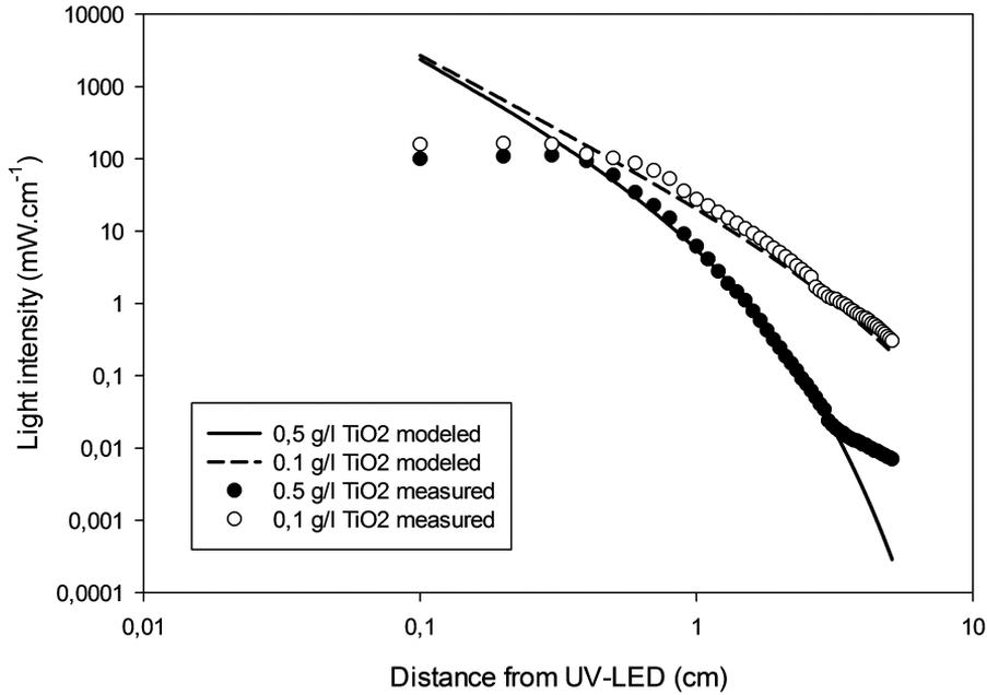
Figure 5.2: Light intensity measurement and modeled of 250 mW UV-LED in a TiO<sub>2</sub> suspension of 0.5 and 0.1 g l<sup>-1</sup>
