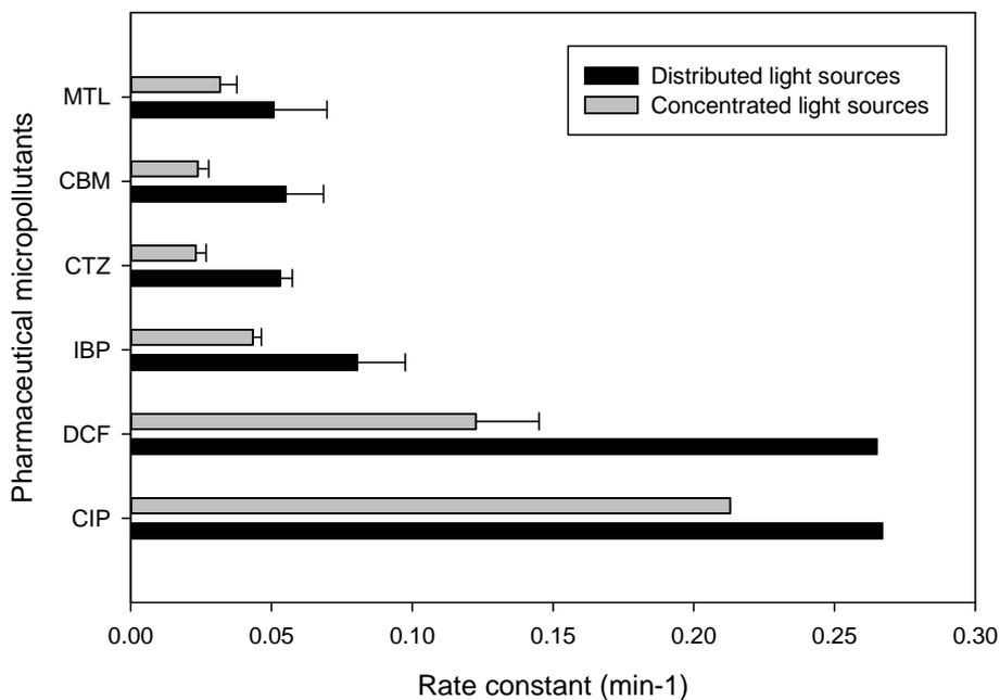
Figure 7.3: Rate constants for removal of pharmaceutical micropollutants from deionized water with distributed and concentrated UV-LEDs, error bars indicate 95% confidence interval.
