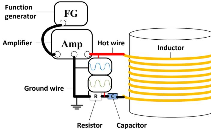
Figure 4.2: Schematic drawing of the transmitting circuit with the function generator and amplifier as the AC source, the inductor, capacitor, resistor and oscilloscope. The hot wire is the wire with non-zero potential.
