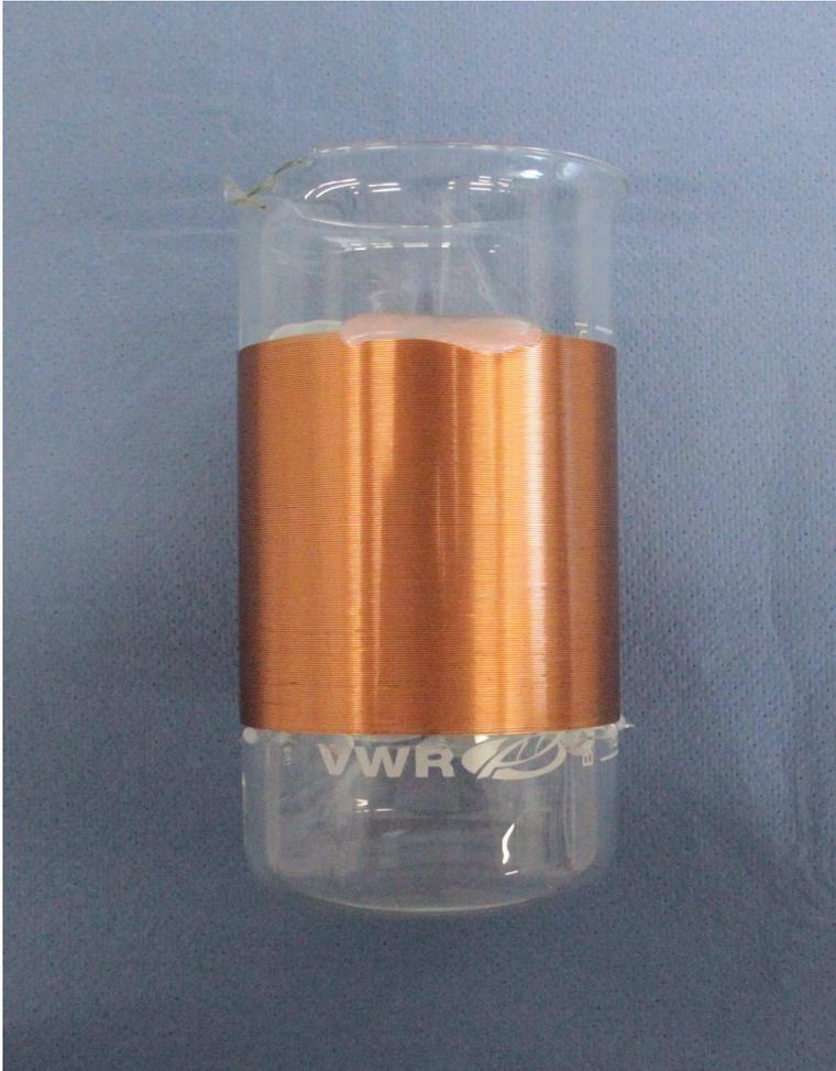
Figure 3.3: Photograph of the inductor around a 1 liter glass beaker.
