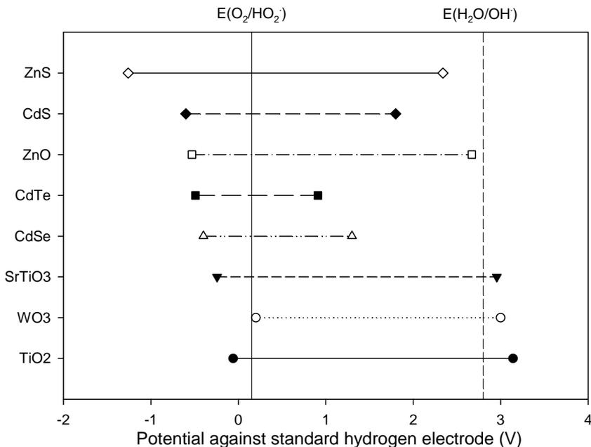
Figure 1.2: Band positions of common n-type semiconductors used in photocatalysis, and the redox potential of  $\text{H}_2\text{O}/\text{OH}\bullet$  and  $\text{O}_2/\text{HO}_2\bullet$  redox couples (data from [130]).
