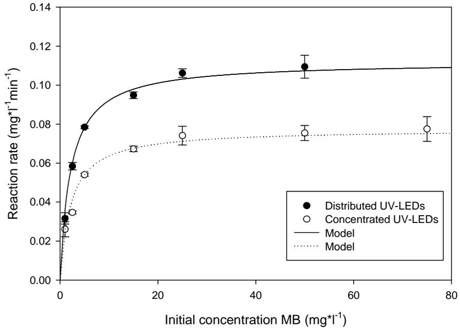
Figure 6.3: Reaction rate as a function of initial concentration methylene blue (MB). Model lines are Langmuir Hinshelwood fits.
