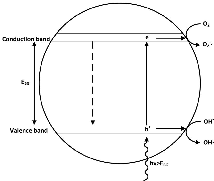
Figure 1.1: Schematic representation of the excitation of an electron from the valence band to the conduction band in the photocatalyst particle and the recombination (dotted line) or the redox reactions on the surface of the particle.
