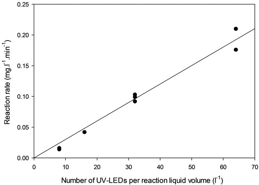
Figure 6.5: Reaction rate as function of number of UV-LEDs per reaction liquid volume.
