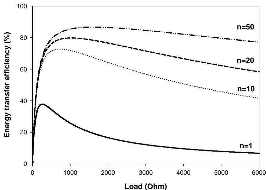
Figure 2.7: Energy transfer efficiency as function of the resistance of the receiving circuit's load, with  $n = 1, 10, 20$  and  $50$  receiving inductors.
