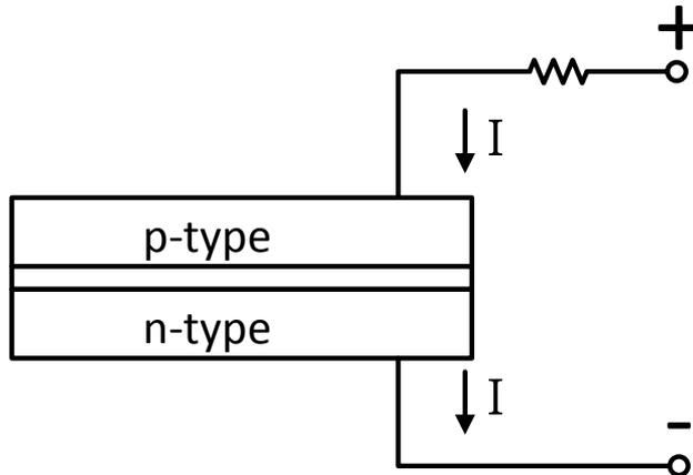
Figure 1.8: A schematic drawing of a light emitting diode with a p and n-type material with current ( $I$ ) flowing from the p-type to the n-type material.
