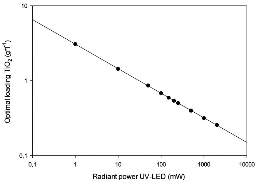
Figure 5.4: Optimal loading as function of the radiant power of the UV-LED
