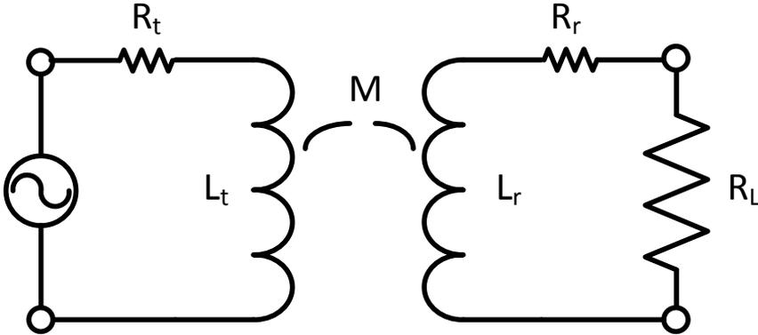
Figure 1.10: Lumped element model of two inductively coupled inductors.
