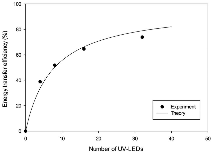
Figure 6.8: Energy transfer efficiency as a function of the number of UV-LEDs.
