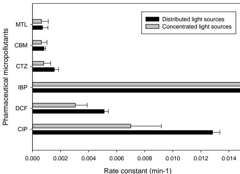
Figure 7.4: Rate constants for removal of pharmaceutical micropollutants from MBR effluent with distributed and concentrated UV-LEDs, error bars indicate 95% confidence interval.
