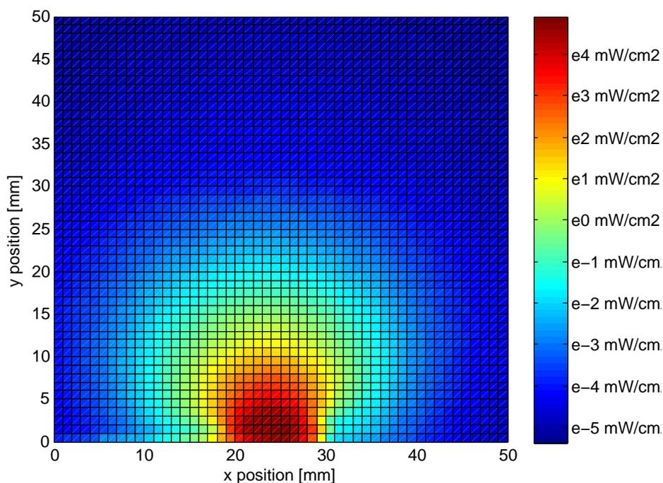
Figure 5.1: Light intensity measurement of 250 mW UV-LED in a  $\text{TiO}_2$  suspension of  $0.5 \text{ gl}^{-1}$
