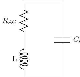
Figure 3.1: Basic lumped equivalent circuit of an inductor.
