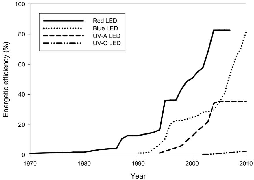
Figure 1.7: Energetic efficiencies of different LEDs over the years
