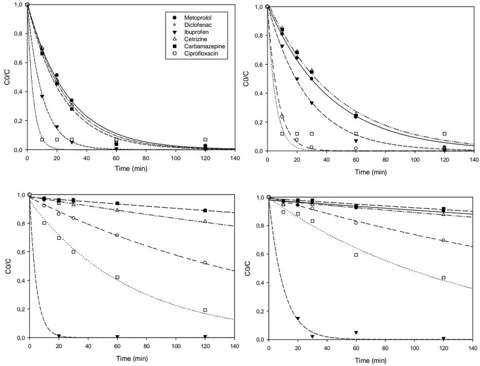
Figure 7.2: The start concentration ( $C_0$ ) over the concentration in time ( $C$ ) as a function of time of six pharmaceuticals with distributed (a) and concentrated (b) UV-LEDs in deionized water and with distributed (c) and concentrated (d) UV-LEDs in MBR effluent.
