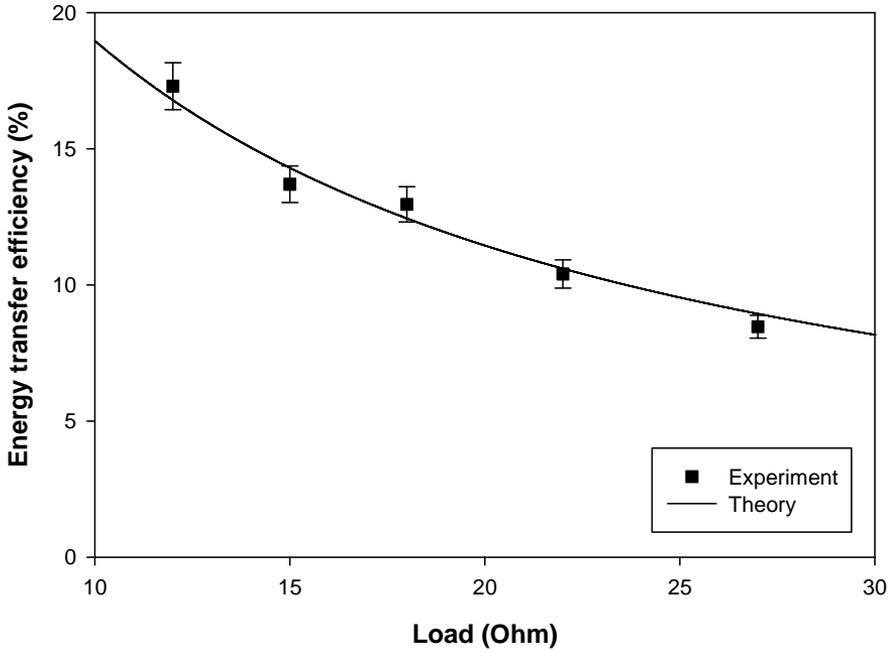
Figure 2.5: Energy transfer efficiency measured and calculated (Equation 2.1) between one transmitting inductor coupled to one receiving inductor with differences in load.
