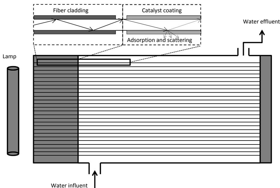
Figure 1.6: Optical fiber reactor with the light source on the left irradiating into the optical fiber and the optical fibers distributing the light over coated catalyst.
