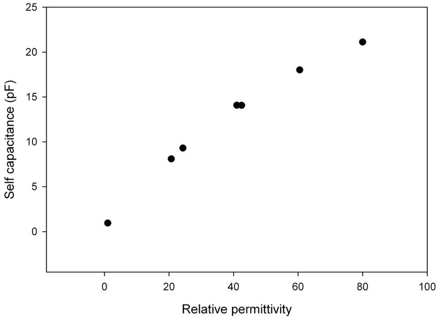
Figure 3.4: Self-capacitance of inductor filled with liquids with difference in relative permittivity.
