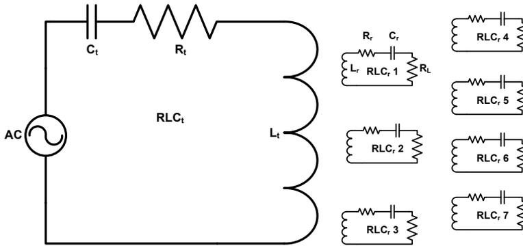
Figure 2.2: Schematic model of 1 transmitting RLC ( $RLC_t$ ) circuit and  $n = 7$  receiving RLC ( $RLC_r$ ) circuits.
