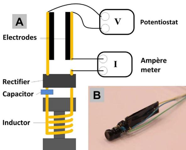
Figure 4.3: (A) Schematic drawing of the receiving circuit combined with two electrodes coated with porous carbon. (B) Photograph of the receiving circuit and two parallel carbon electrodes used for wireless water desalination.
