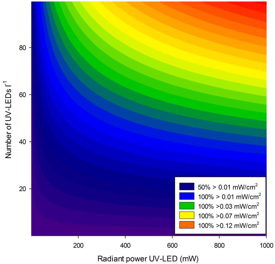
Figure 6.7: Contour plot showing the efficiency of illumination as a function of number of UV-LEDs per liter and the radiant power of the UV-LEDs.
