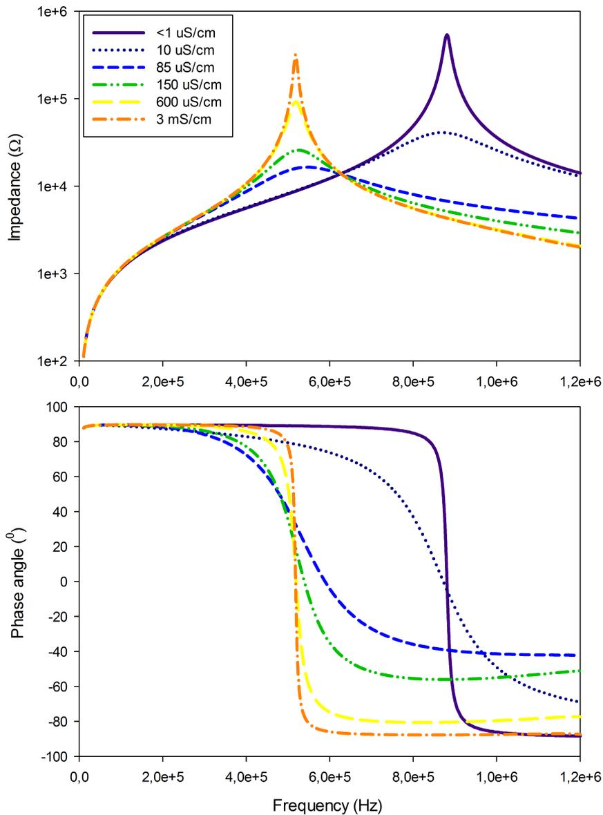
Figure 3.6: Impedance and phase angle as a function of frequency for inductor wound around the glass beaker, filled with water/ethanol mixture with different conductivities.
