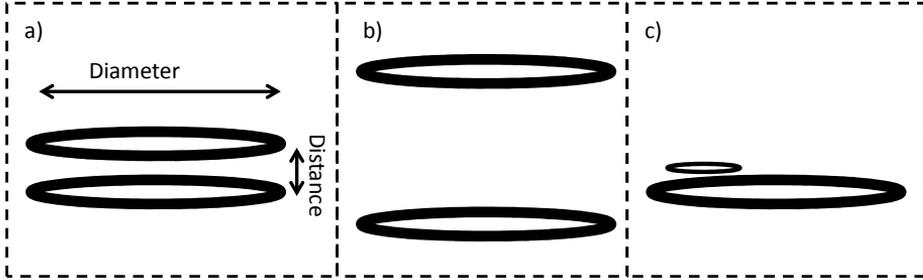
Figure 1.9: Schematic drawing of (a) inductors tightly coupled, (b) loosely coupled inductors with increased distance between the inductors and (c) loosely coupled inductors with difference in diameter.
