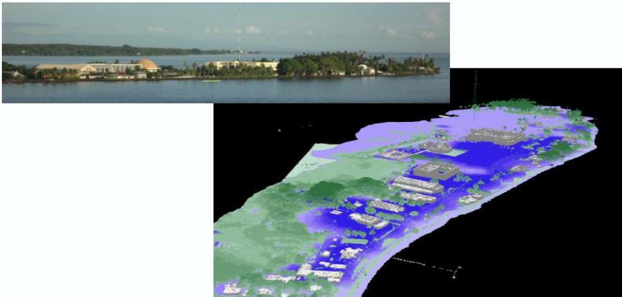
*Tide+surge (IBE+wind setup)+wave setup+ runup*
