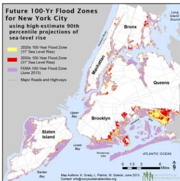
The potential areas that could be impacted by the 100-year flood in the 2020s and 2050s based on projections of the high-estimate 90th percentile sea level rise scenario
