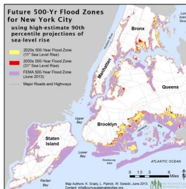
The potential areas that could be impacted by the 500-year flood in the 2020s and 2050s based on projections of the high-estimate 90th percentile sea level rise scenario
