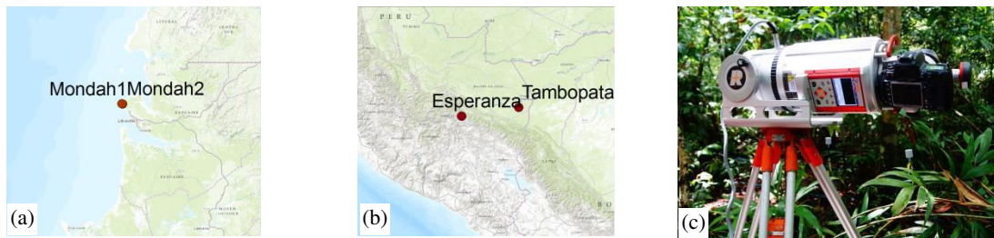
Figure 1. Study area and data acquisition. (a) shows Mondah1 and Mondah2 plots, located in Gabon, Africa; while (b) shows Tambopata and Esperanza plots in Peru, South America. RIEGL VZ-400V-Line 3D ® TLS in tilted scan configuration can be seen in (c).
