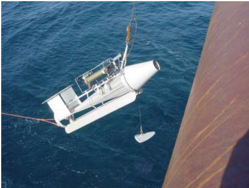
Figure 3.1. The Gulf VII plankton sampler.
