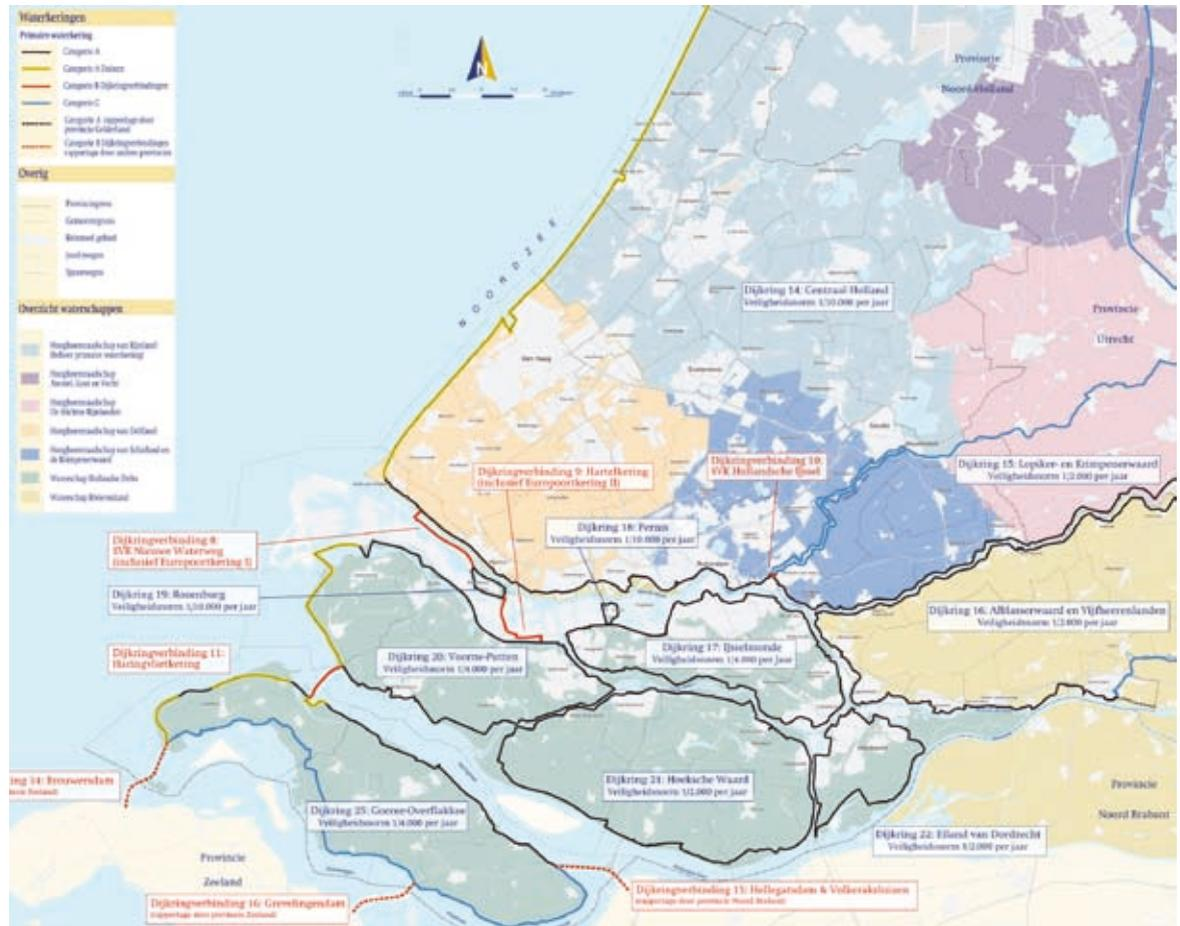
Figure 17: Dike rings and dike ring links in the west Netherlands
