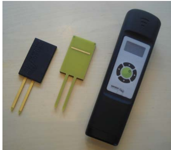
Fig. 1: The AquaTag system, with reader and sensor tags.
