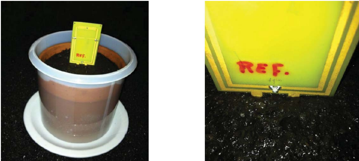
Fig. 5: AquaTag sensor in earthenware pot with compost (left) and detail (right).
