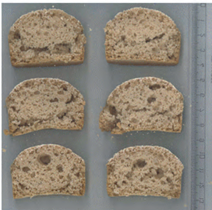
Figure 9. Crumb appearance of bread slices of oat flour with or without WPP. Incorporation of WPP improved crumb texture at both consistencies tested. The picture shows the bread slices made at 500 BU consistency: (a) pure oat flour; (b) oat flour/WPP.
